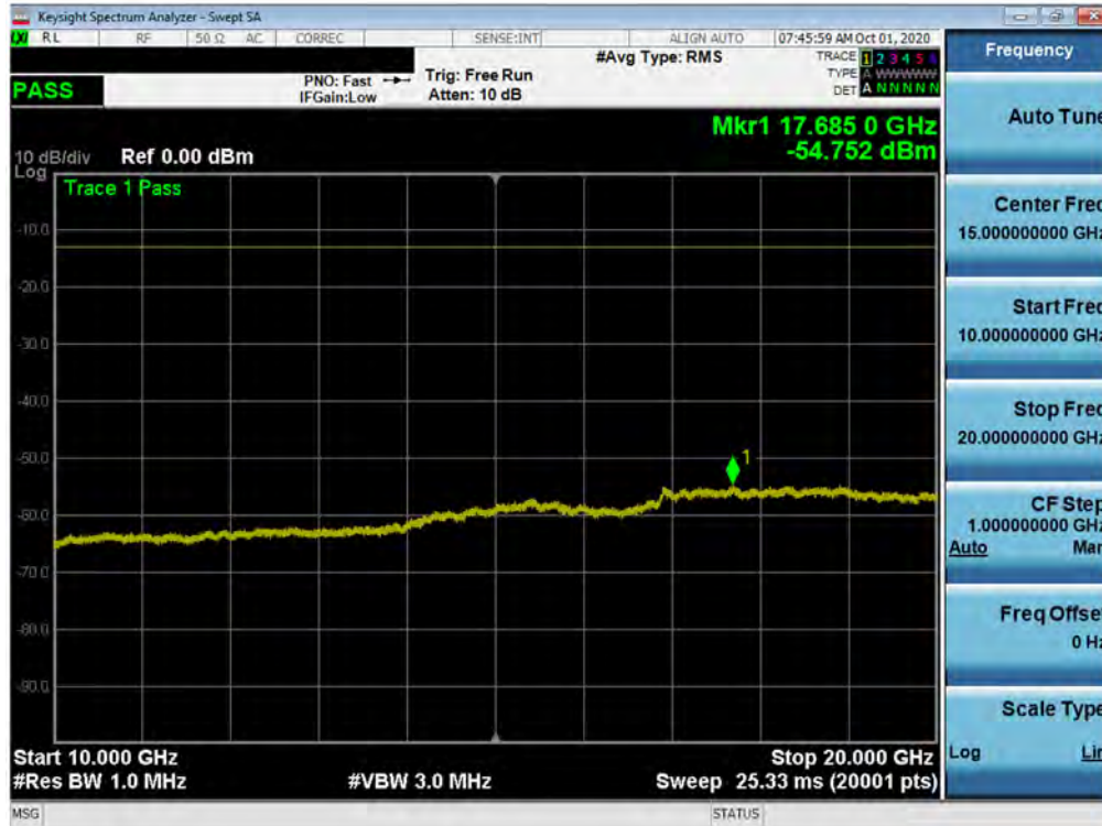
Plot 7-110. Conducted Spurious Plot (NR Band n25/n2 - 20.0MHz - RB Size 1, RB Offset 0 - Low Channel)
