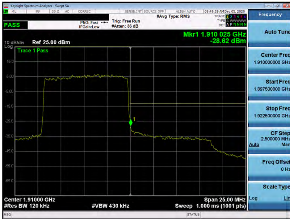
Plot 7-236. Upper Band Edge Plot (NR Band n2 - 10.0MHz - Full RB)
