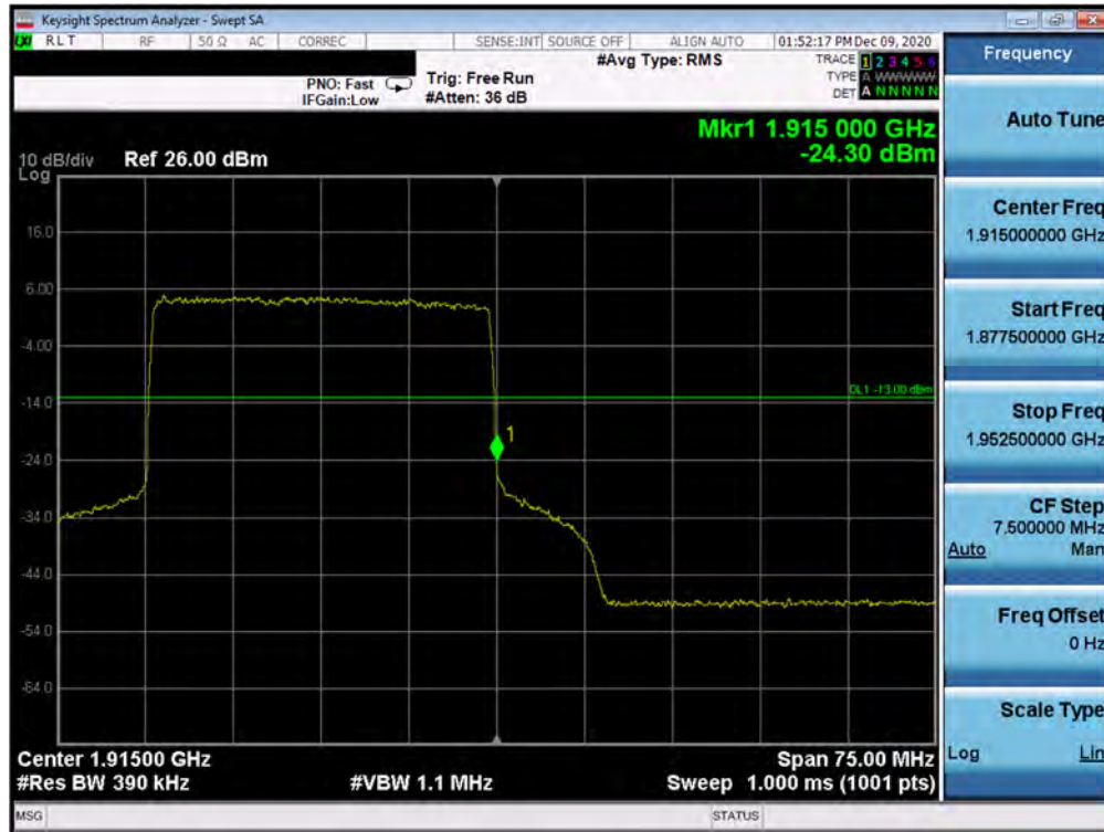
Plot 7-180. Upper Band Edge Plot (NR Band n25 - 30.0MHz - Full RB)
