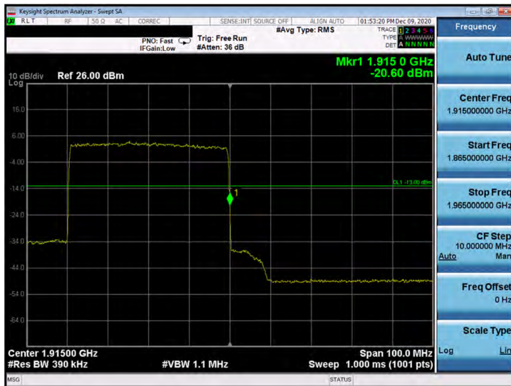
Plot 7-176. Upper Band Edge Plot (NR Band n25 - 40.0MHz - Full RB)
