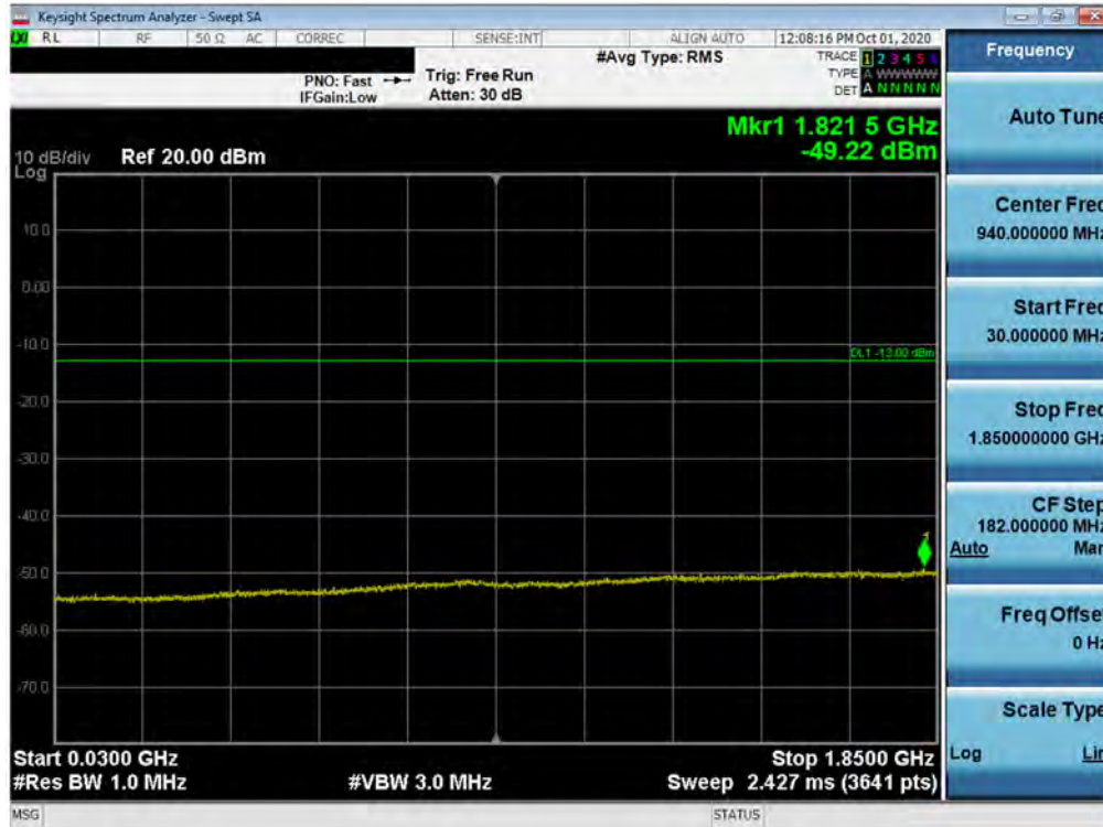
Plot 7-105. Conducted Spurious Plot (LTE Band 25/2 - 20MHz QPSK - RB Size 1, RB Offset 0 - High Channel)
