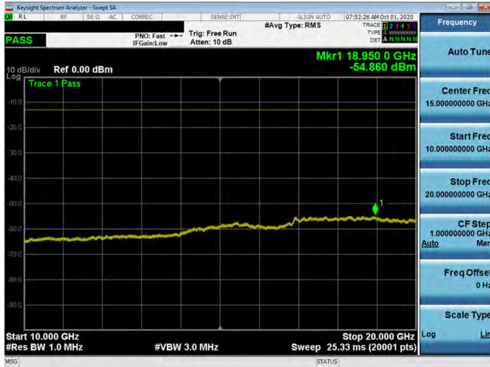
Plot 7-116. Conducted Spurious Plot (NR Band n25/n2 - 20.0MHz - RB Size 1, RB Offset 0 - High Channel)
