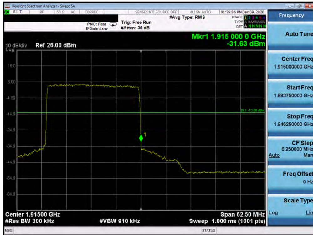
Plot 7-220. Upper Band Edge Plot (NR Band n25 - 25.0MHz - Full RB)
