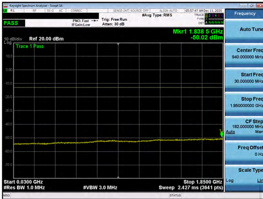
Plot 7-120. Conducted Spurious Plot (NR Band n25/n2 - 20.0MHz - RB Size 1, RB Offset 0 - Mid Channel)
