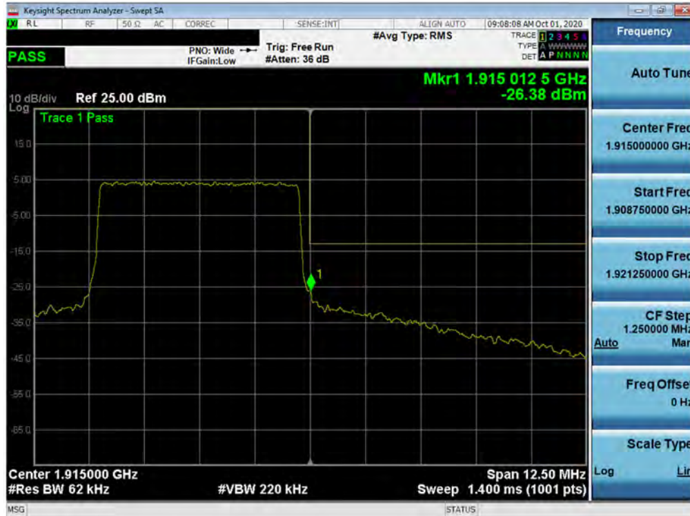
Plot 7-208. Upper Band Edge Plot (NR Band n25 – 5.0MHz - Full RB)
