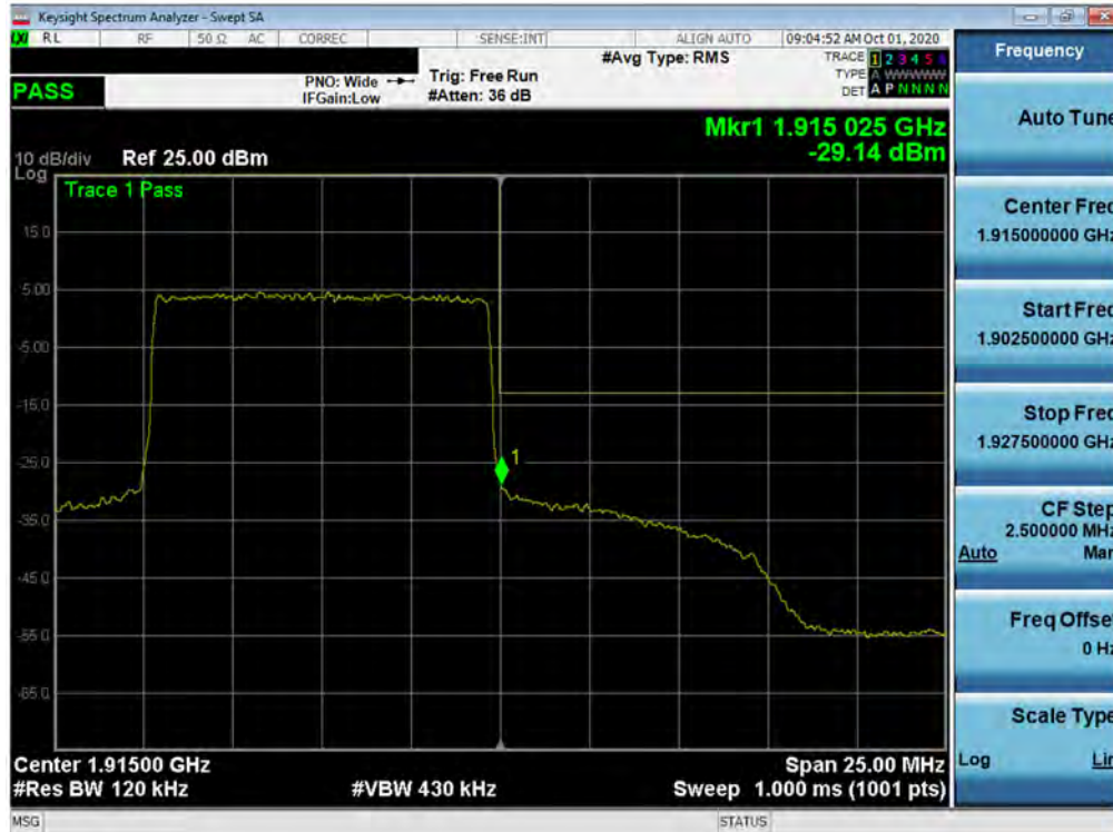
Plot 7-202. Upper Band Edge Plot (NR Band n25 – 10.0MHz - Full RB)
