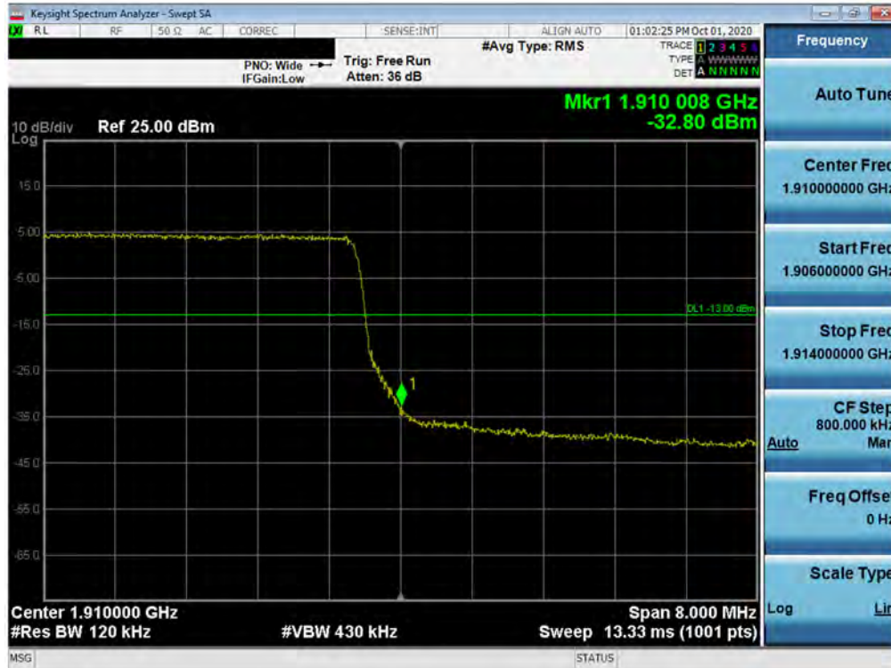
Plot 7-152. Upper Band Edge Plot (LTE Band 2 - 10MHz QPSK – Full RB Configuration)
