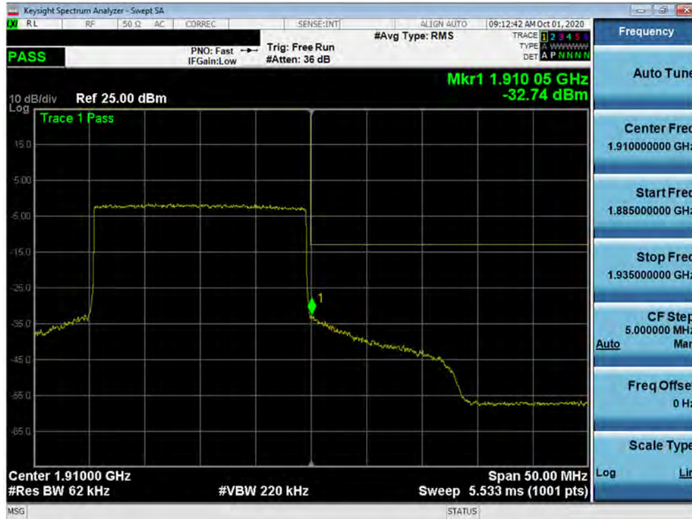
Plot 7-190. Upper Band Edge Plot (NR Band n2 – 20.0MHz - Full RB)
