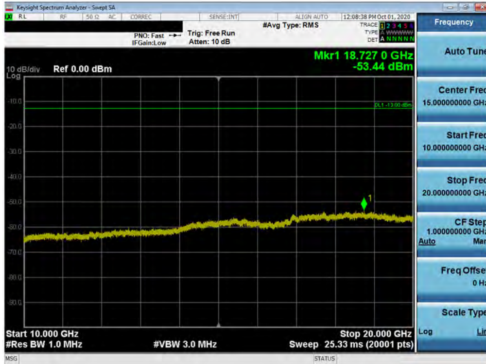
Plot 7-107. Conducted Spurious Plot (LTE Band 25/2 - 20MHz QPSK - RB Size 1, RB Offset 0 - High Channel)
