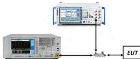
Figure 7-4. Test Instrument & Measurement Setup
