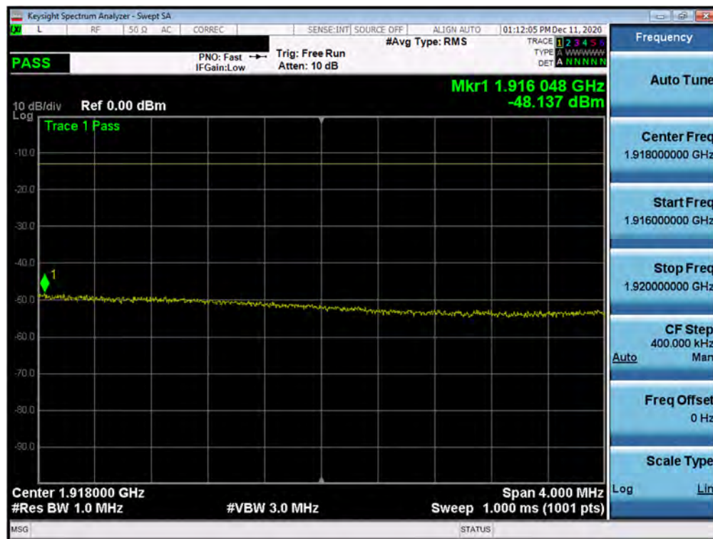
Plot 7-227. Upper Extended Band Edge Plot (NR Band n25 – 20.0MHz - Full RB)
