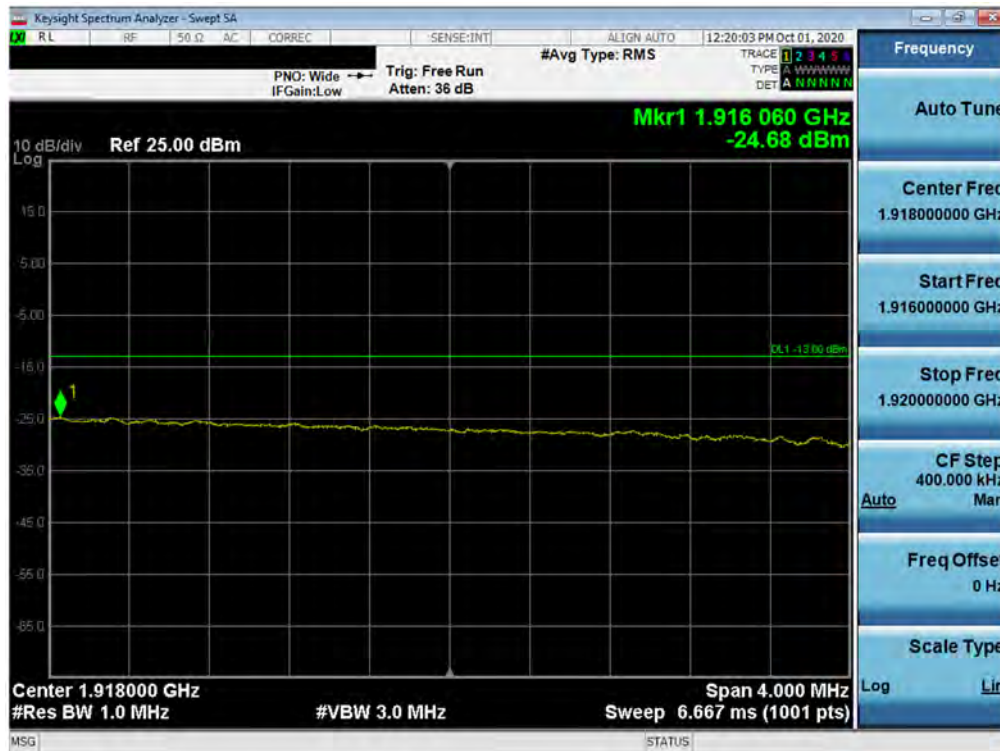
Plot 7-149. Extended Upper Band Edge Plot (LTE Band 25 - 15MHz QPSK – Full RB Configuration)
