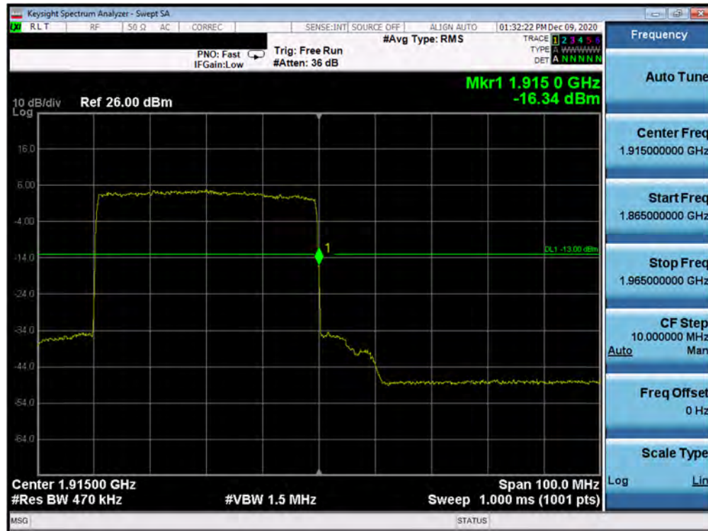
Plot 7-212. Upper Band Edge Plot (NR Band n25 – 40.0MHz - Full RB)
