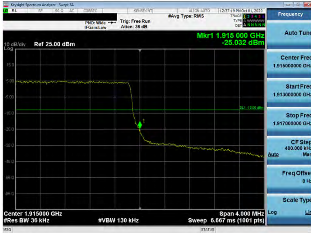
Plot 7-166. Upper Band Edge Plot (LTE Band 25 - 3MHz QPSK – Full RB Configuration)
