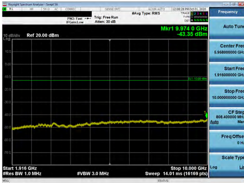
Plot 7-106. Conducted Spurious Plot (LTE Band 25/2 - 20MHz QPSK - RB Size 1, RB Offset 0 - High Channel)
