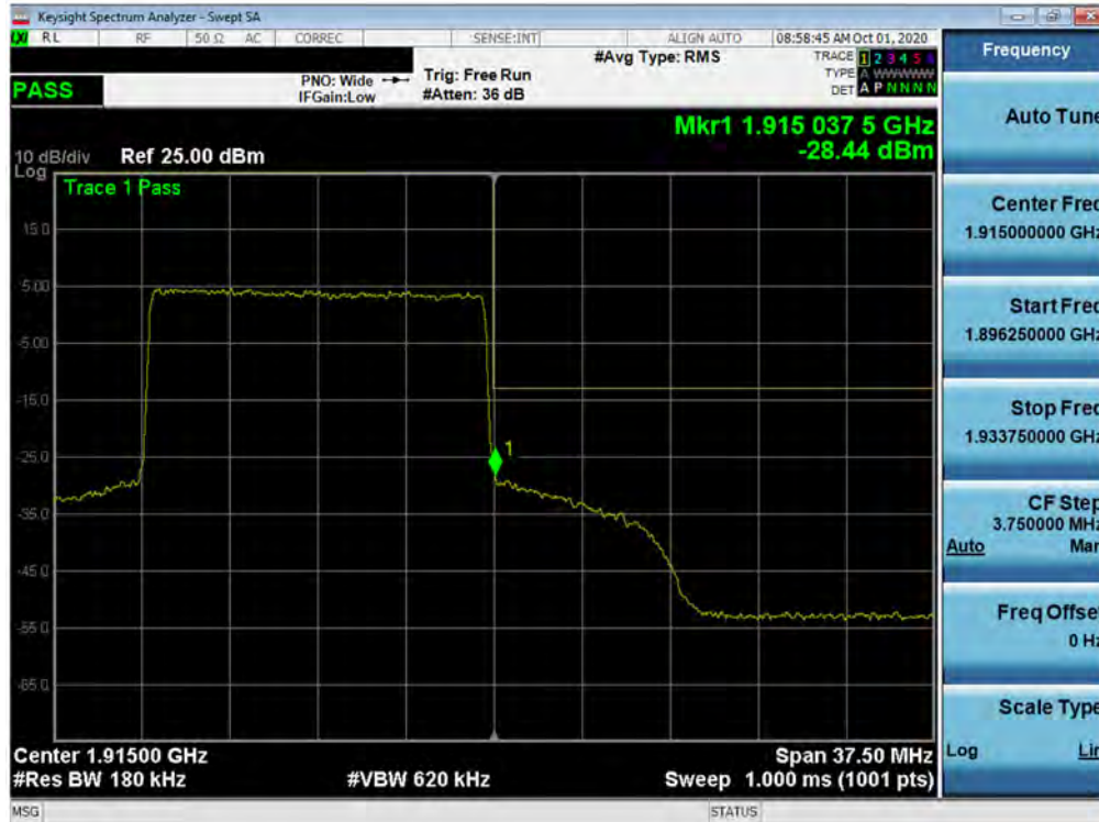
Plot 7-194. Upper Band Edge Plot (NR Band n25 – 15.0MHz - Full RB)
