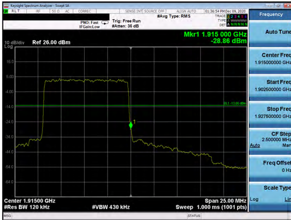
Plot 7-238. Upper Band Edge Plot (NR Band n25 – 10.0MHz - Full RB)
