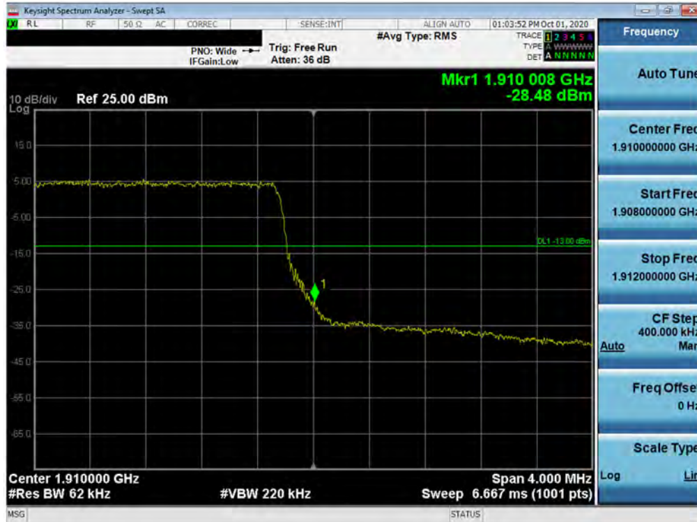
Plot 7-158. Upper Band Edge Plot (LTE Band 2 - 5MHz QPSK – Full RB Configuration)
