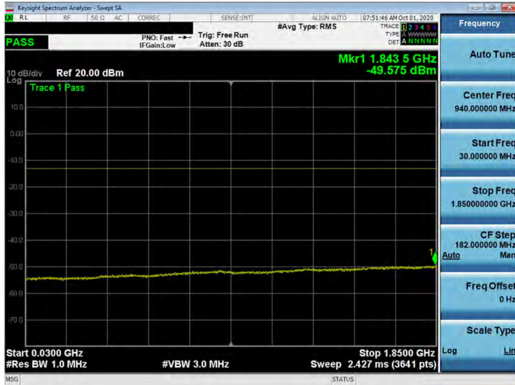
Plot 7-114. Conducted Spurious Plot (NR Band n25/n2 - 20.0MHz - RB Size 1, RB Offset 0 - High Channel)
