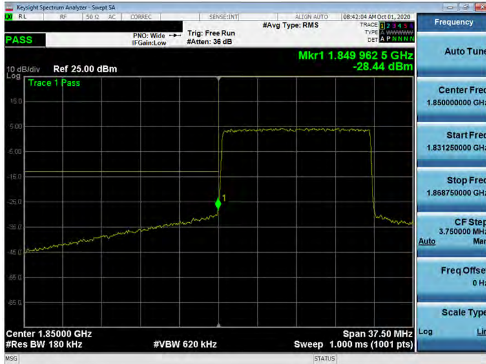
Plot 7-192. Lower Band Edge Plot (NR Band n25/2 – 15.0MHz - Full RB)
