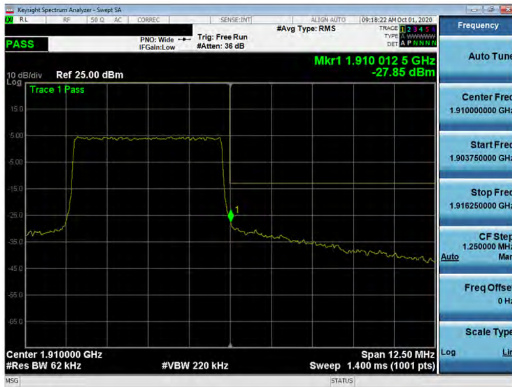
Plot 7-206. Upper Band Edge Plot (NR Band n2 – 5.0MHz - Full RB)
