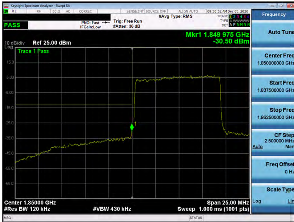
Plot 7-234. Lower Band Edge Plot (NR Band n25/2 – 10.0MHz - Full RB)
