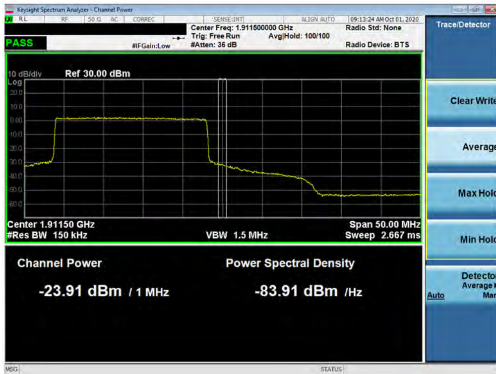
Plot 7-191. Upper Extended Band Edge Plot (NR Band n2 – 20.0MHz - Full RB)
