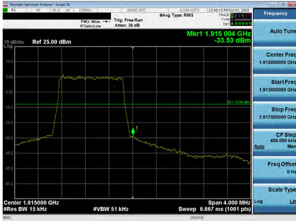
Plot 7-172. Upper Band Edge Plot (LTE Band 25 – 1.4MHz QPSK – Full RB Configuration)
