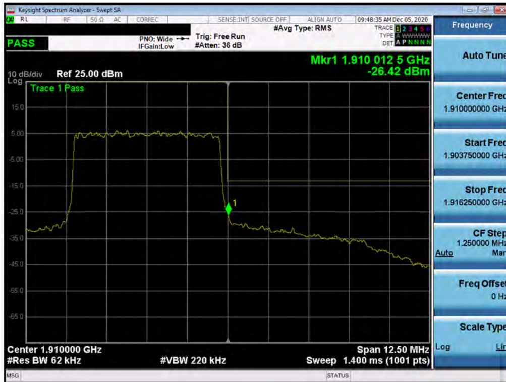
Plot 7-242. Upper Band Edge Plot (NR Band n2 – 5.0MHz - Full RB)
