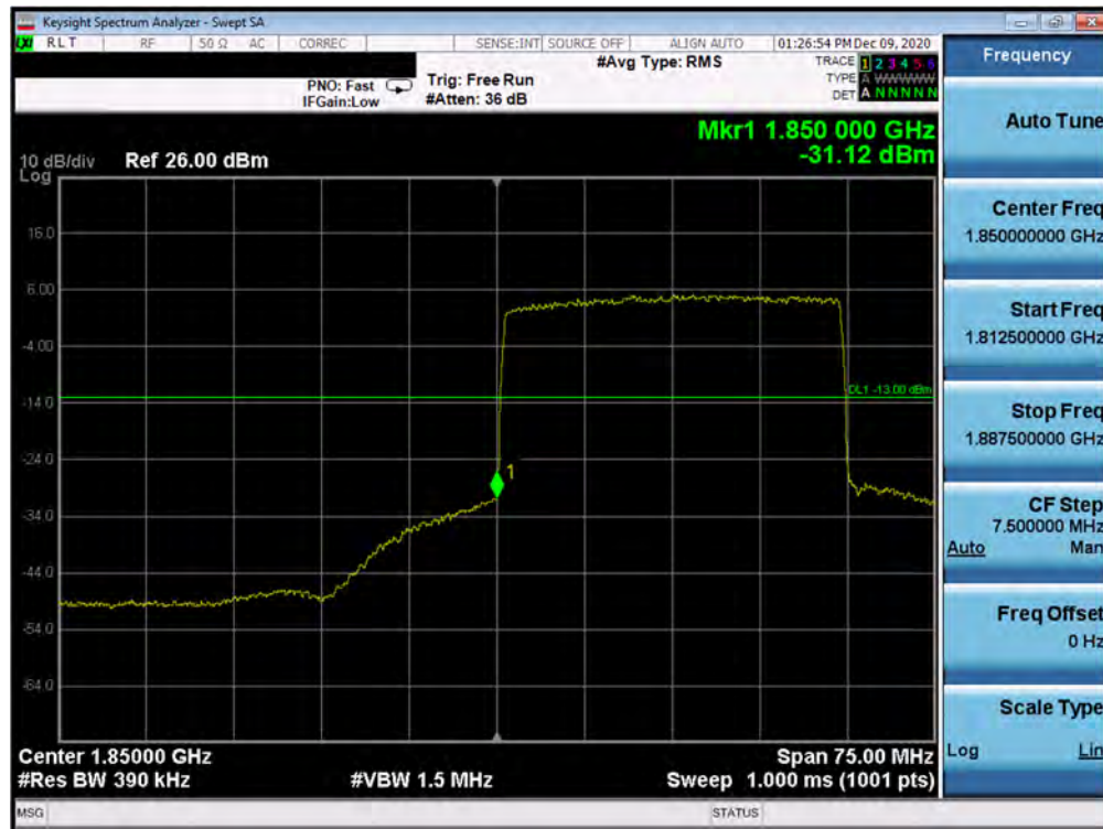
Plot 7-214. Lower Band Edge Plot (NR Band n25 – 30.0MHz - Full RB)
