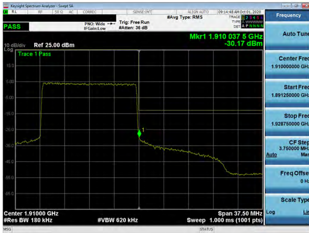
Plot 7-196. Upper Band Edge Plot (NR Band n2 – 15.0MHz - Full RB)
