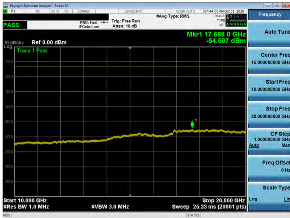
Plot 7-113. Conducted Spurious Plot (NR Band n25/n2 - 20.0MHz - RB Size 1, RB Offset 0 - Mid Channel)
