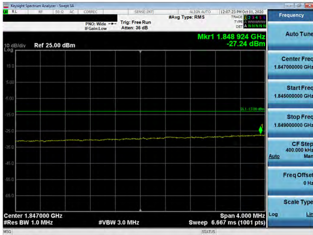
Plot 7-139. Extended Lower Band Edge Plot (LTE Band 25/2 - 20MHz QPSK – Full RB Configuration)
