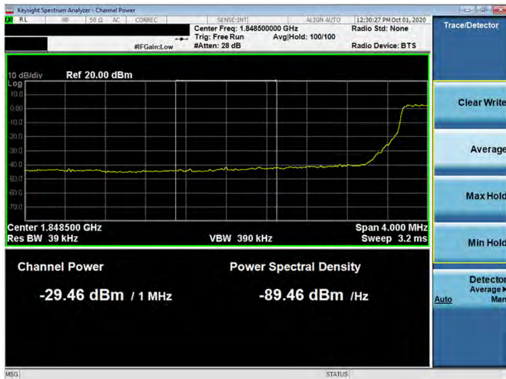
Plot 7-157. Extended Lower Band Edge Plot (LTE Band 25/2 - 5MHz QPSK – Full RB Configuration)
