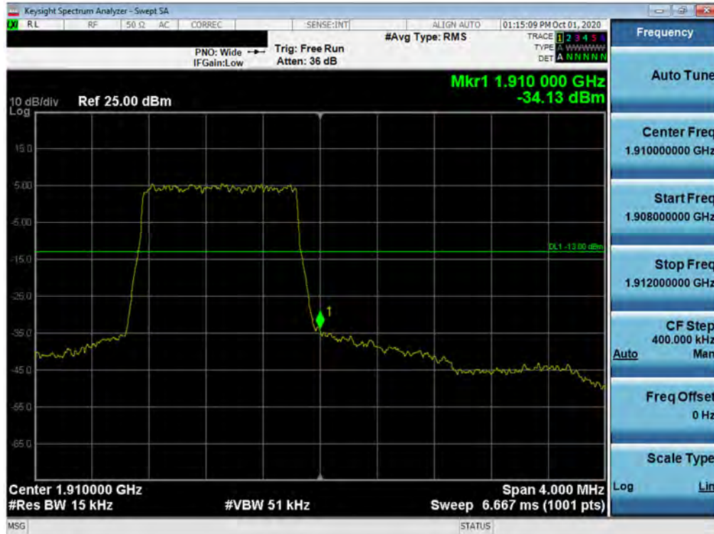
Plot 7-170. Upper Band Edge Plot (LTE Band 2 – 1.4MHz QPSK – Full RB Configuration)
