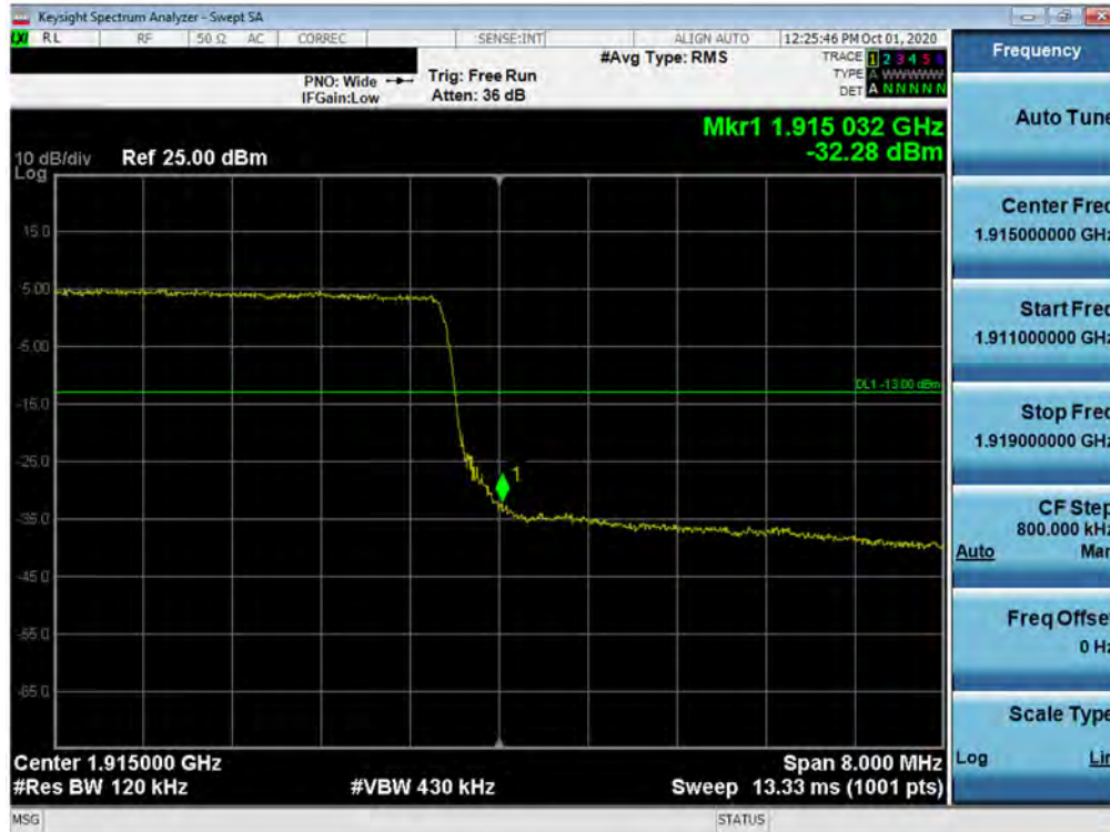
Plot 7-154. Upper Band Edge Plot (LTE Band 25 - 10MHz QPSK – Full RB Configuration)
