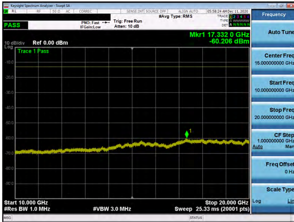
Plot 7-119. Conducted Spurious Plot (NR Band n25/n2 - 20.0MHz - RB Size 1, RB Offset 0 - Low Channel)
