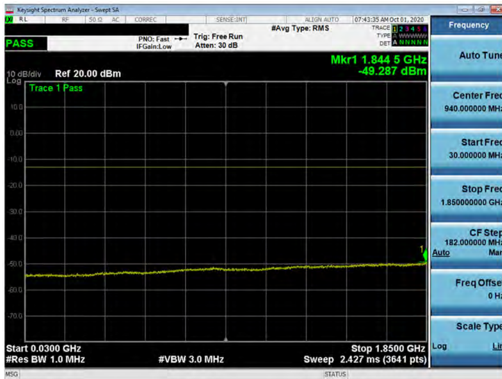
Plot 7-111. Conducted Spurious Plot (NR Band n25/n2 - 20.0MHz - RB Size 1, RB Offset 0 - Mid Channel)
