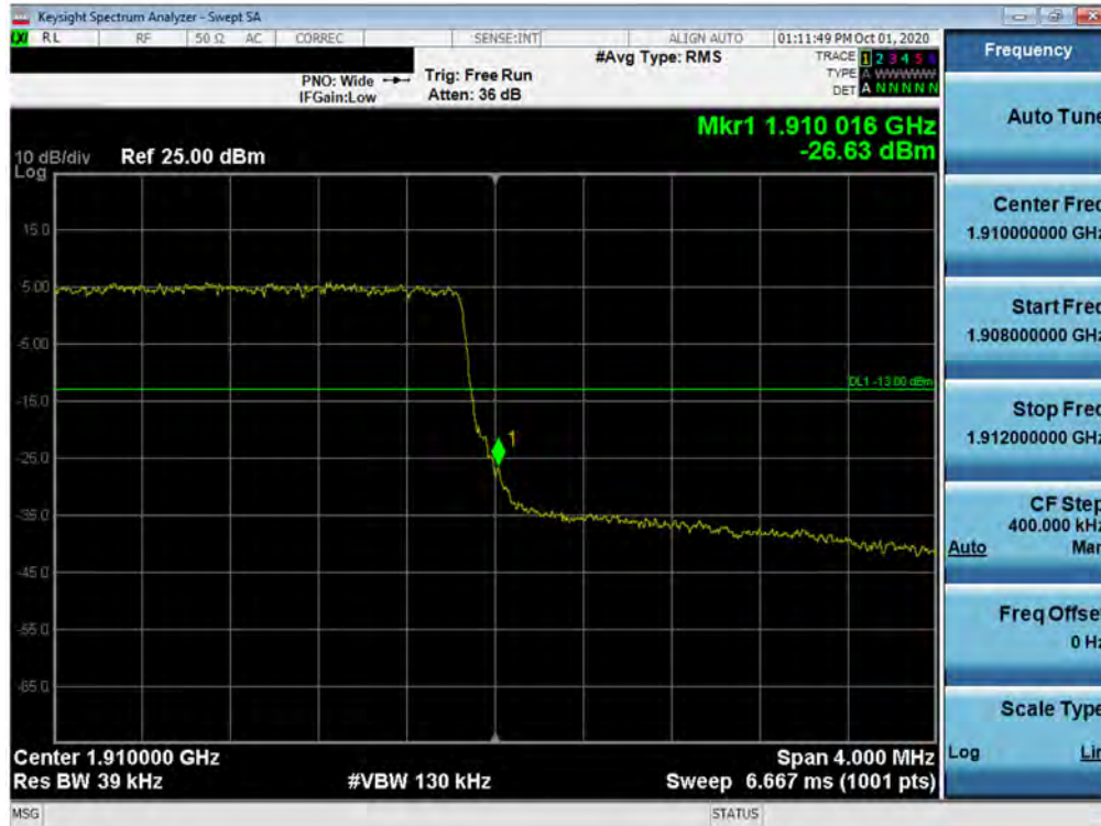
Plot 7-164. Upper Band Edge Plot (LTE Band 2 - 3MHz QPSK – Full RB Configuration)
