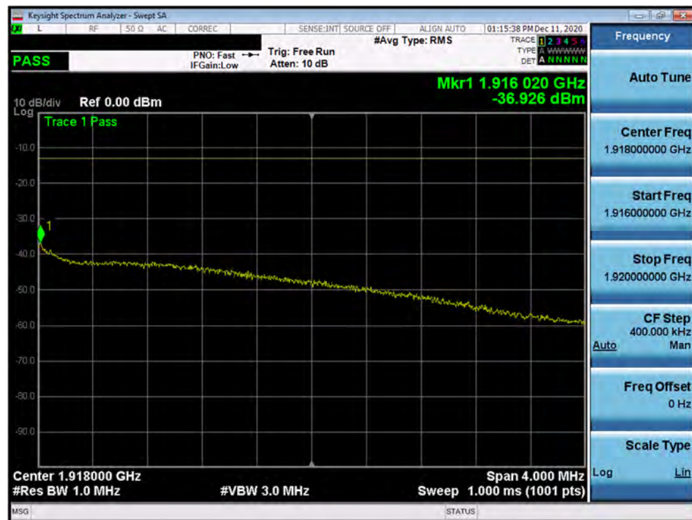
Plot 7-245. Upper Extended Band Edge Plot (NR Band n25 - 5.0MHz - Full RB)
