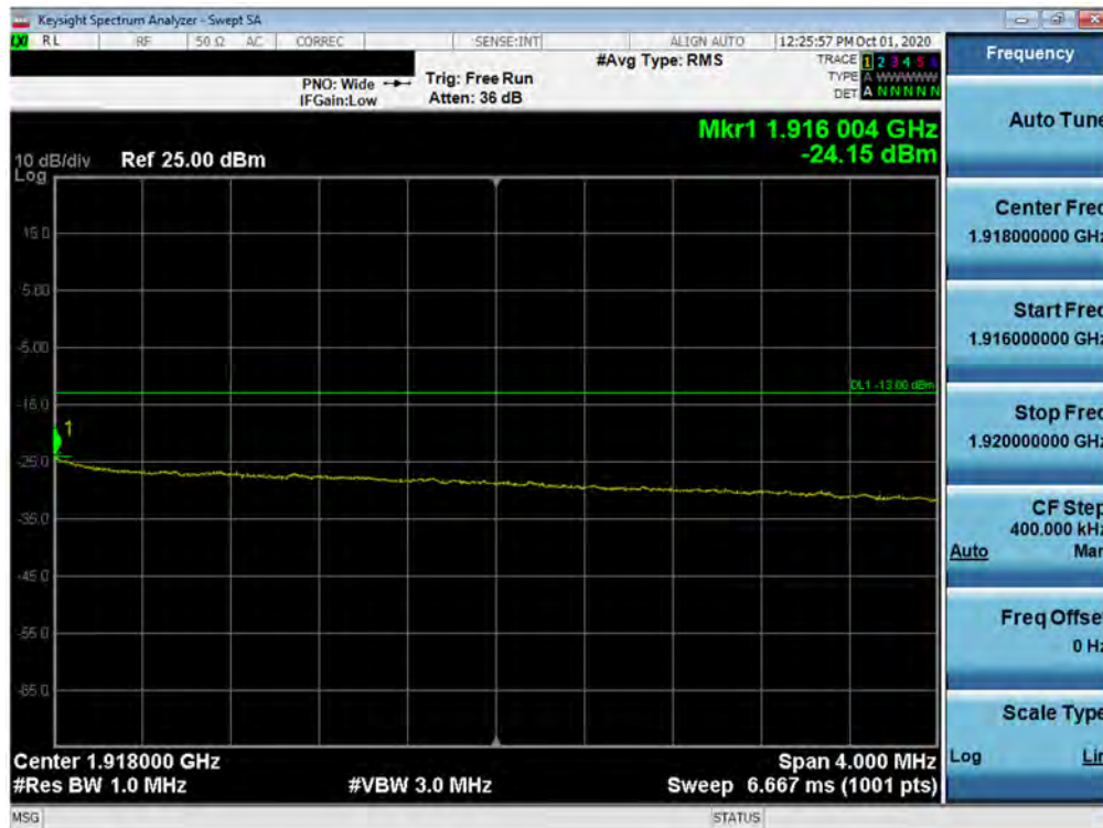
Plot 7-155. Extended Upper Band Edge Plot (LTE Band 25 - 10MHz QPSK – Full RB Configuration)
