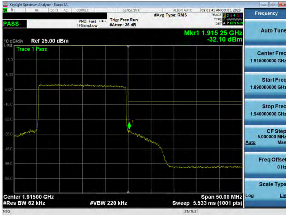
Plot 7-188. Upper Band Edge Plot (NR Band n25 – 20.0MHz - Full RB)
