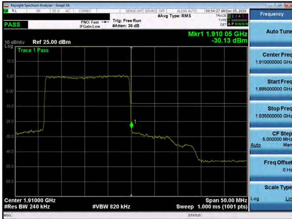
Plot 7-224. Upper Band Edge Plot (NR Band n2 – 20.0MHz - Full RB)
