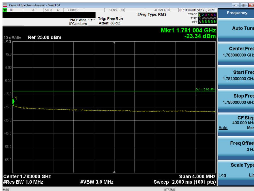
Plot 7-220. Upper Extended Band Edge Plot (LTE Band 66 - 10MHz QPSK – Full RB Configuration)
