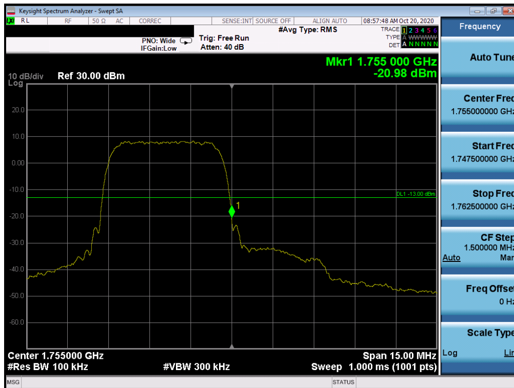
Plot 7-201. Upper Band Edge Plot (WCDMA AWS - Ch. 1513)
