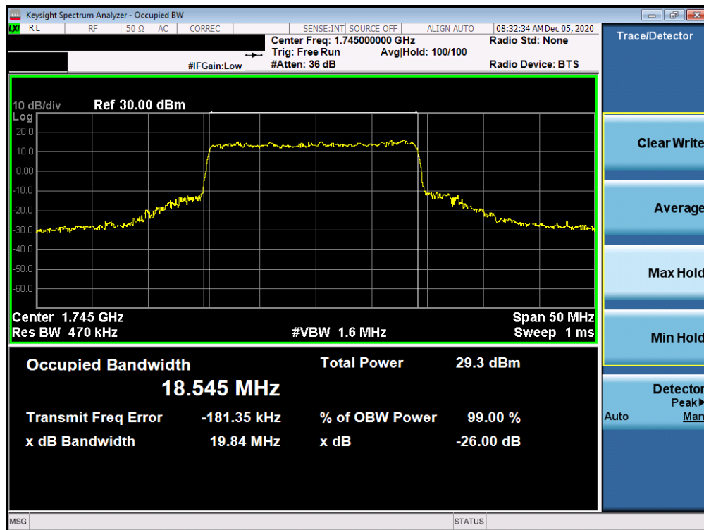
Plot 7-142. Occupied Bandwidth Plot (NR Band n66 - 20.0MHz CP-OFDM QPSK - Full RB)
