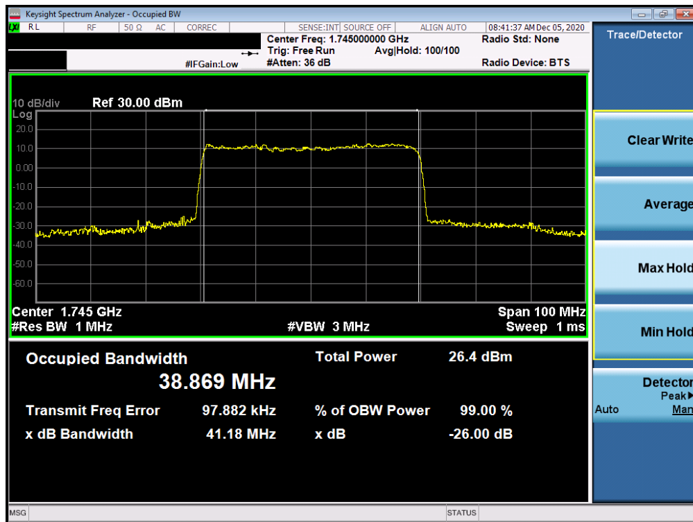
Plot 7-135. Occupied Bandwidth Plot (NR Band n66 - 40.0MHz CP-OFDM 256QAM - Full RB)
