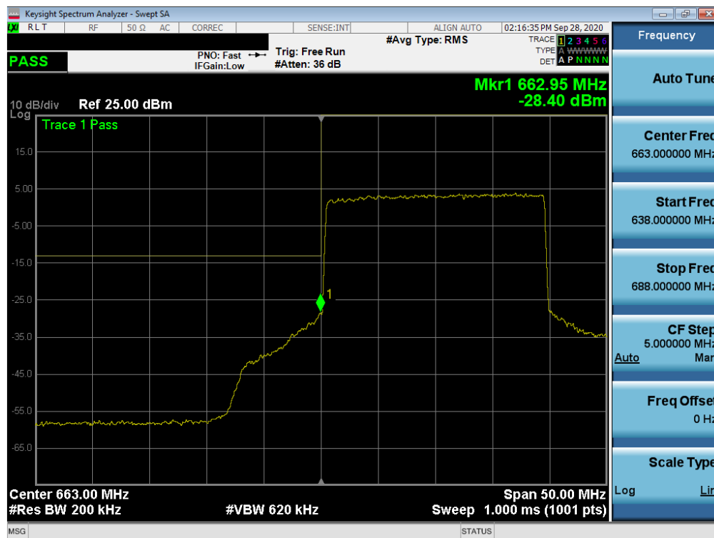
Plot 7-169. Lower Band Edge Plot (NR Band n71 – 20.0MHz - Full RB)
