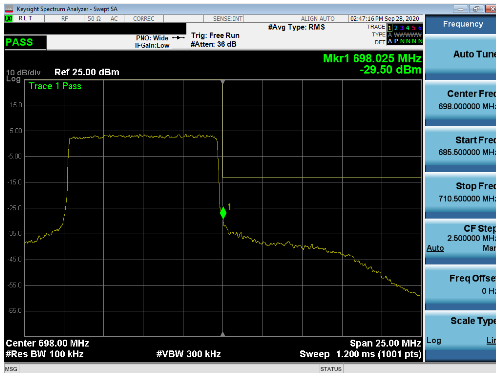
Plot 7-174. Upper Band Edge Plot (NR Band n71 - 10.0MHz - Full RB)
