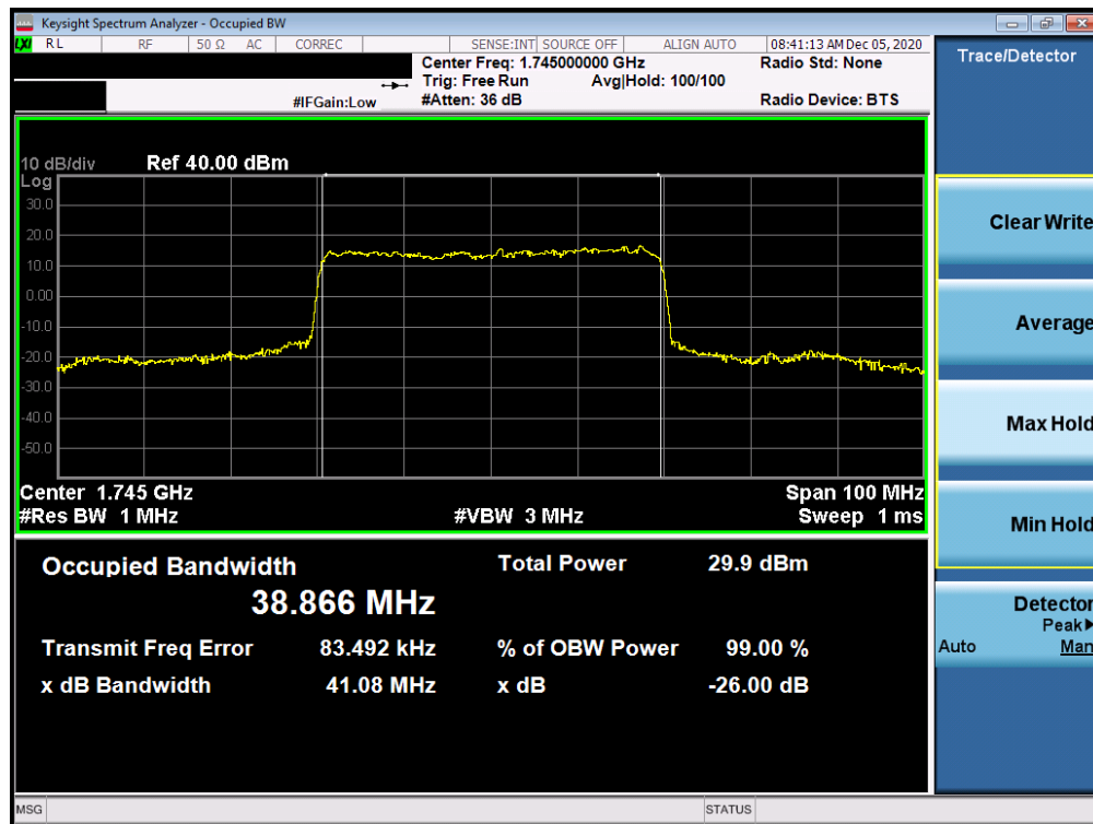
Plot 7-133. Occupied Bandwidth Plot (NR Band n66 - 40.0MHz CP-OFDM 16QAM - Full RB)
