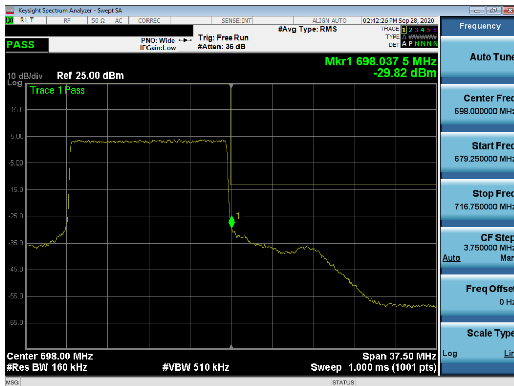
Plot 7-172. Upper Band Edge Plot (NR Band n71 - 15.0MHz - Full RB)
