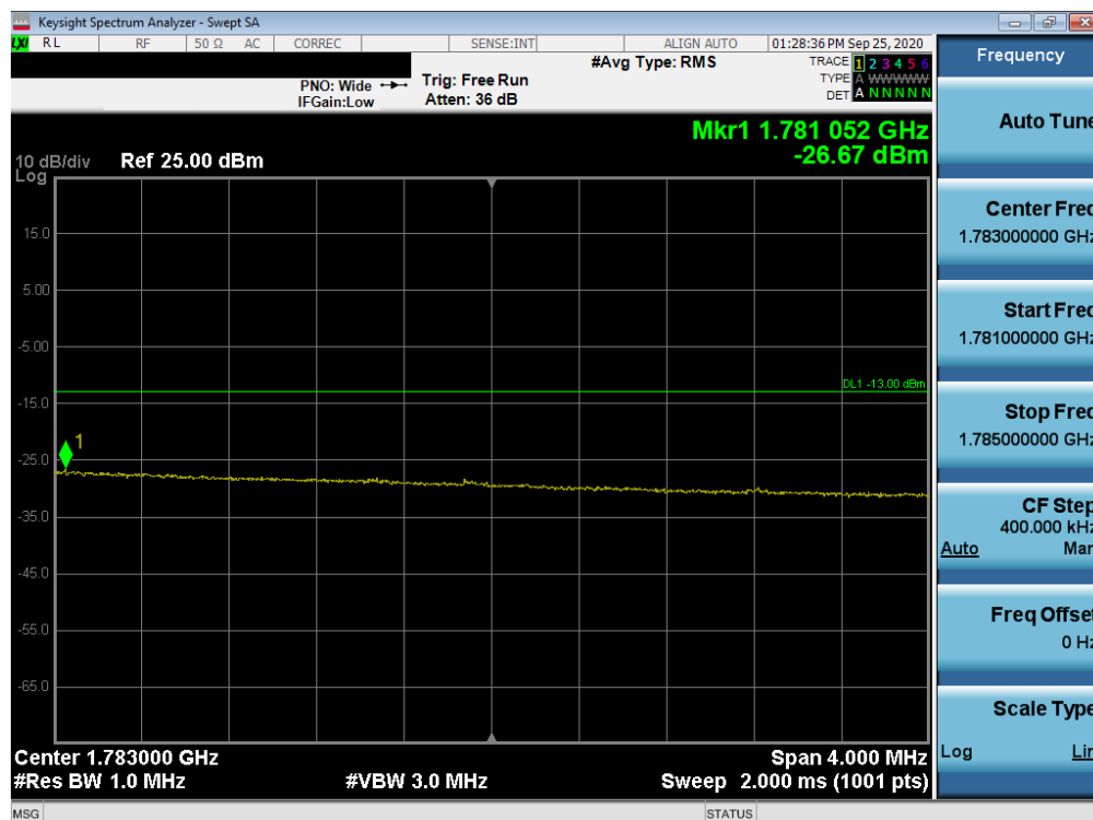
Plot 7-214. Upper Extended Band Edge Plot (LTE Band 66 - 15MHz QPSK – Full RB Configuration)
