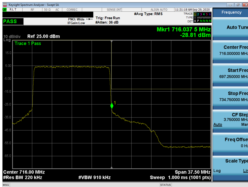
Plot 7-186. Upper Band Edge Plot (NR Band n12 – 15.0MHz - Full RB)
