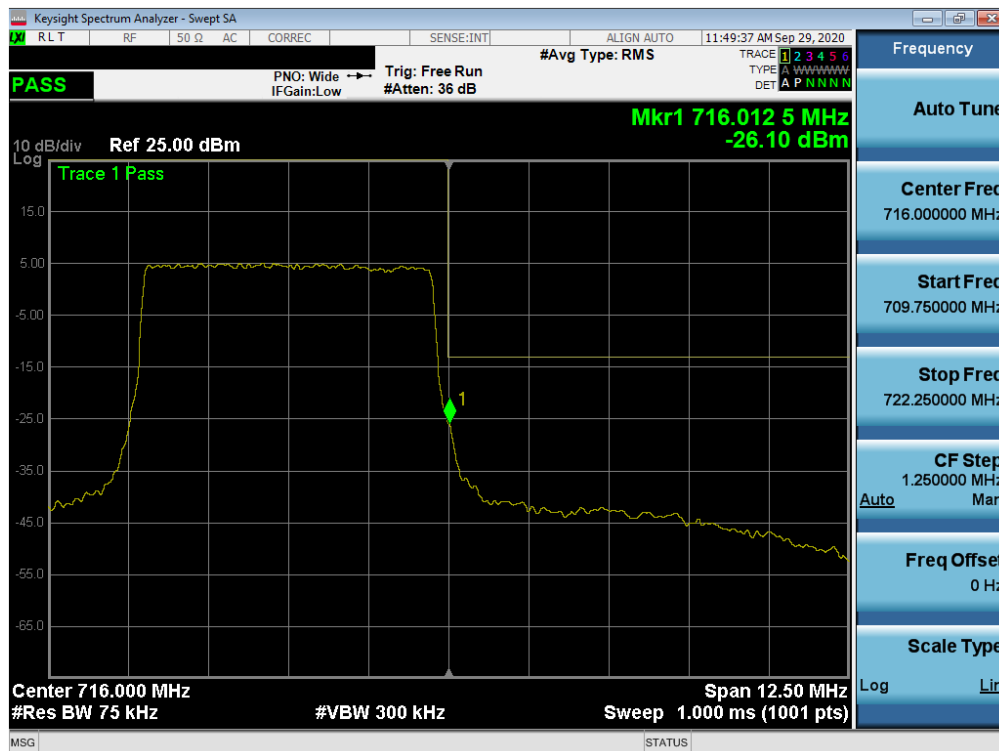
Plot 7-190. Upper Band Edge Plot (NR Band n12 - 5.0MHz - Full RB)
