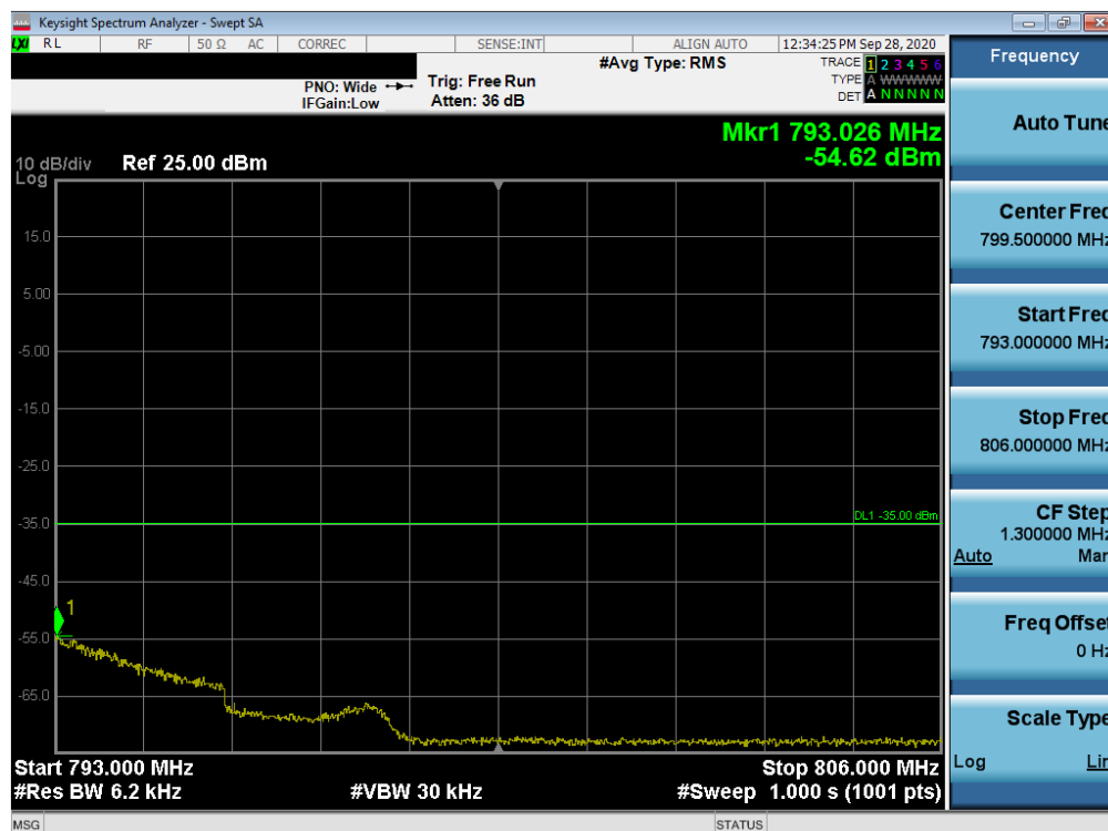
Plot 7-194. Upper Emission Mask Plot (LTE Band 13 - 10MHz QPSK – Full RB Configuration)
