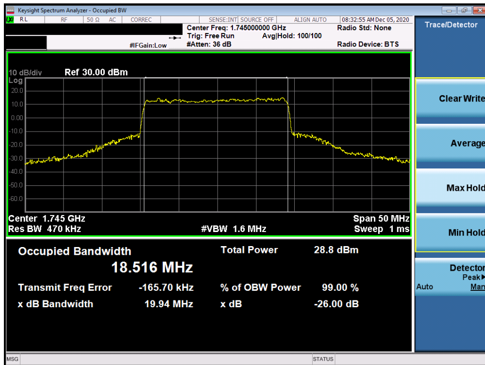
Plot 7-144. Occupied Bandwidth Plot (NR Band n66 - 20.0MHz CP-OFDM 64QAM - Full RB)
