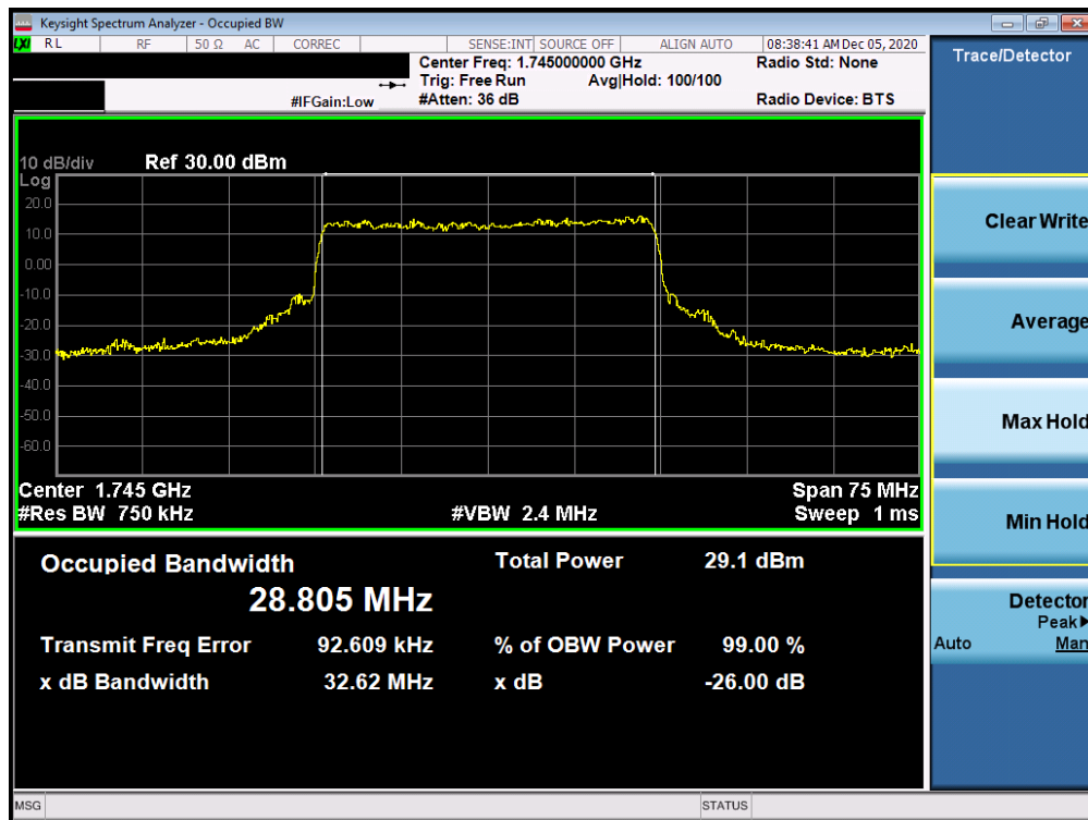
Plot 7-139. Occupied Bandwidth Plot (NR Band n66 - 30.0MHz CP-OFDM 64QAM - Full RB)
