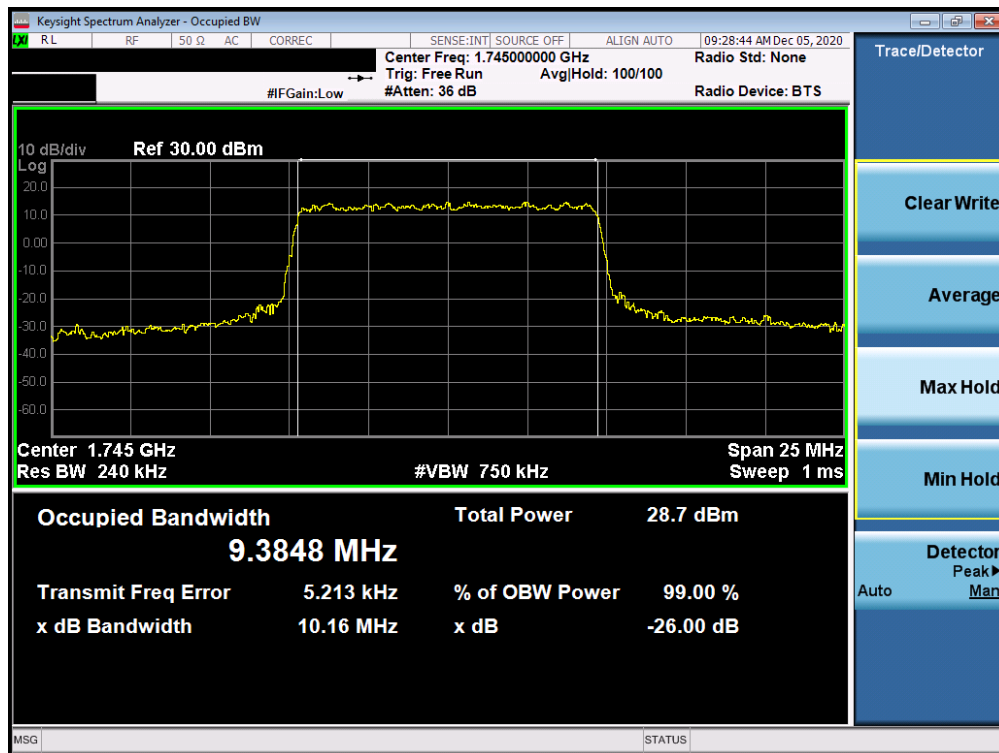
Plot 7-153. Occupied Bandwidth Plot (NR Band n66 - 10.0MHz CP-OFDM 16QAM - Full RB)
