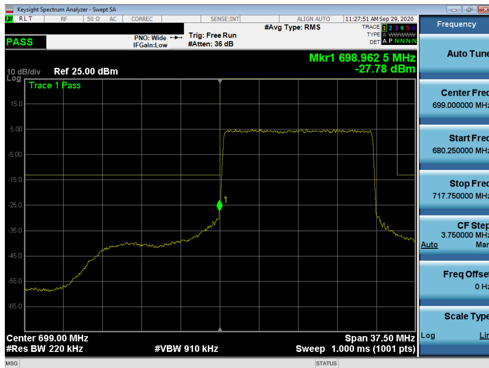
Plot 7-185. Lower Band Edge Plot (NR Band n12 – 15.0MHz - Full RB)
