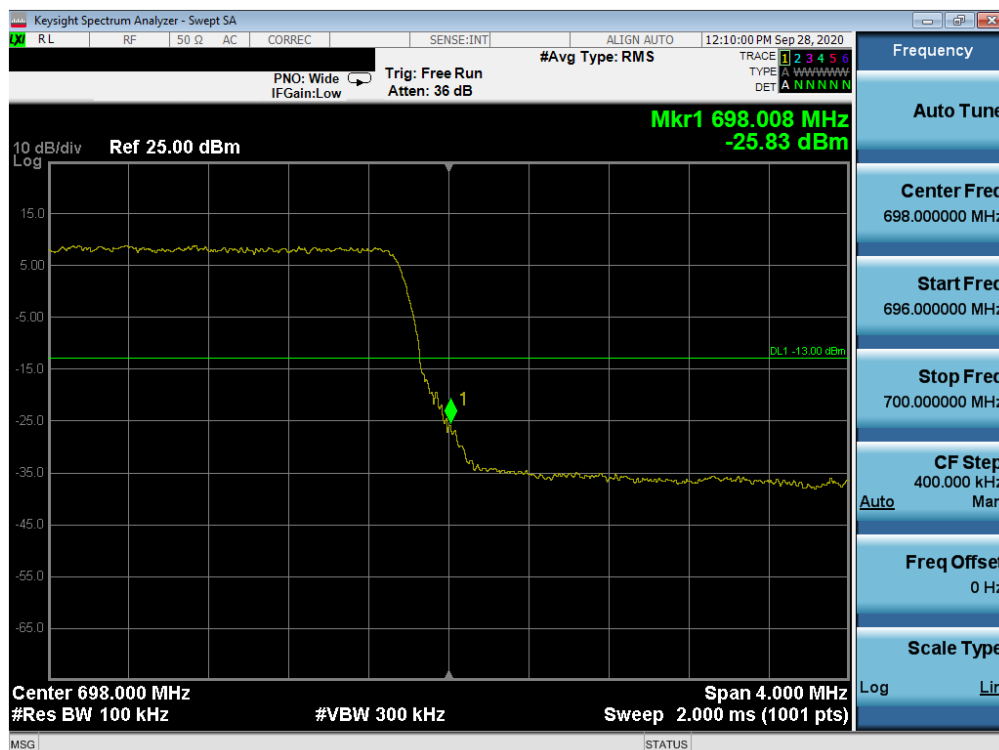
Plot 7-168. Upper Band Edge Plot (LTE Band 71 - 5MHz QPSK – Full RB Configuration)
