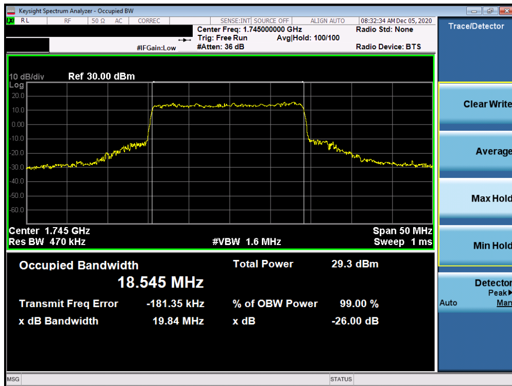
Plot 7-145. Occupied Bandwidth Plot (NR Band n66 - 20.0MHz CP-OFDM 256QAM - Full RB)
