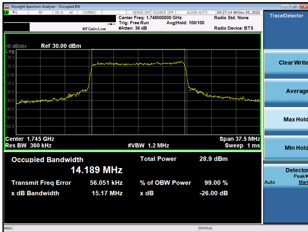
Plot 7-148. Occupied Bandwidth Plot (NR Band n66 - 15.0MHz CP-OFDM 16QAM - Full RB)
