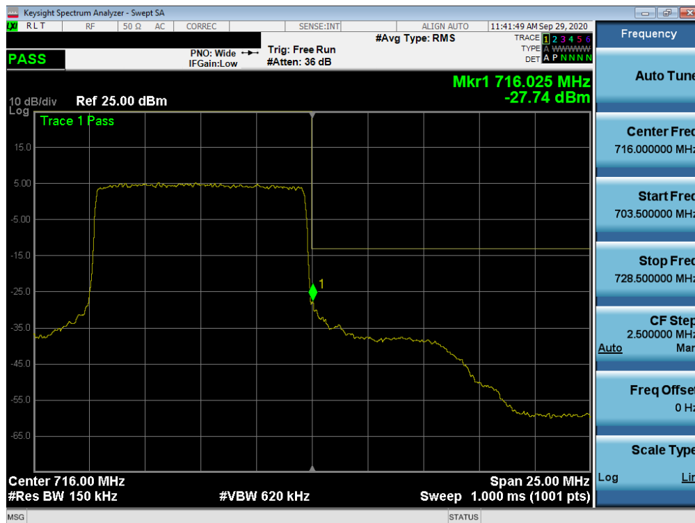
Plot 7-188. Upper Band Edge Plot (NR Band n12 - 10.0MHz - Full RB)
