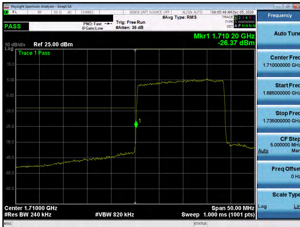
Plot 7-263. Lower Band Edge Plot (NR Band n66 – 20.0MHz - Full RB)
