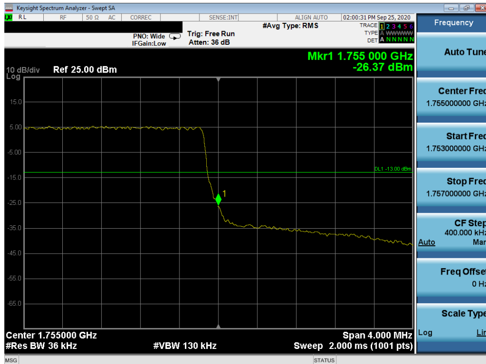
Plot 7-229. Upper Band Edge Plot (LTE Band 4 - 3MHz QPSK – Full RB Configuration)
