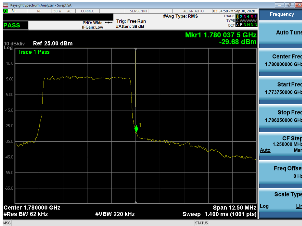
Plot 7-257. Upper Band Edge Plot (NR Band n66 – 5.0MHz - Full RB)
