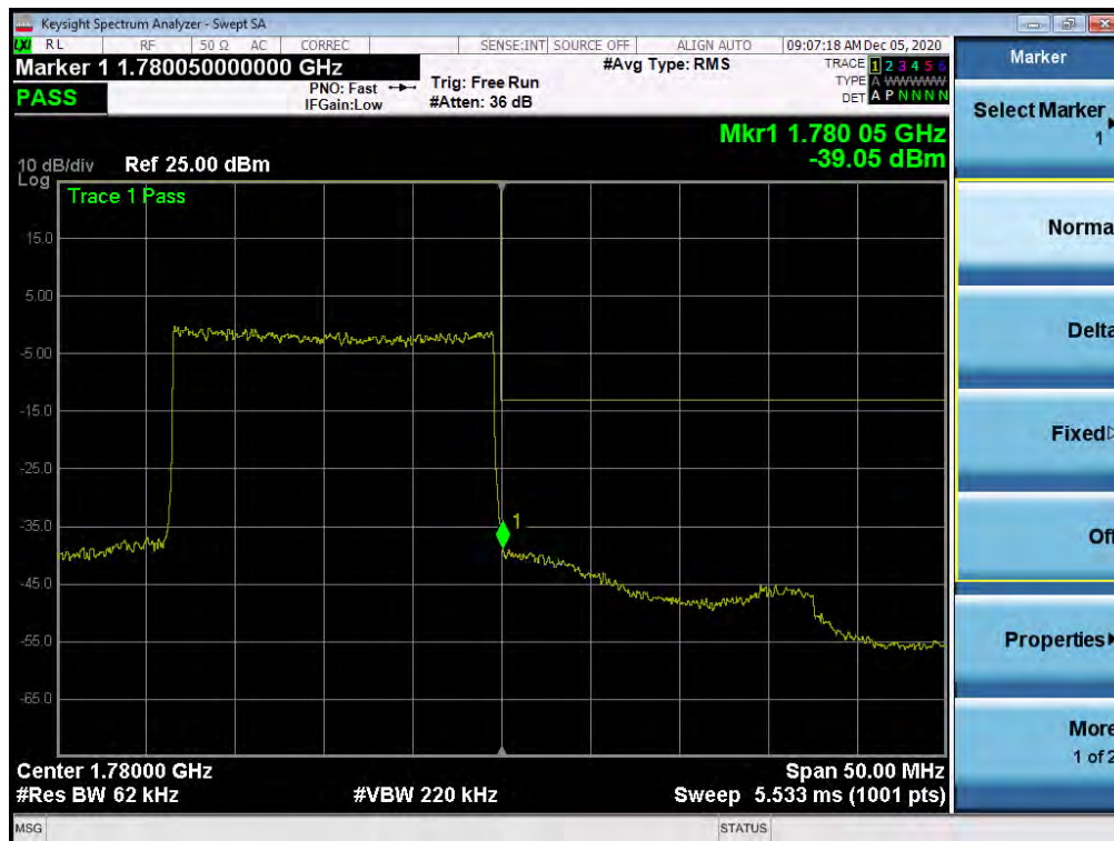
Plot 7-265. Upper Band Edge Plot (NR Band n66 – 20.0MHz - Full RB)
