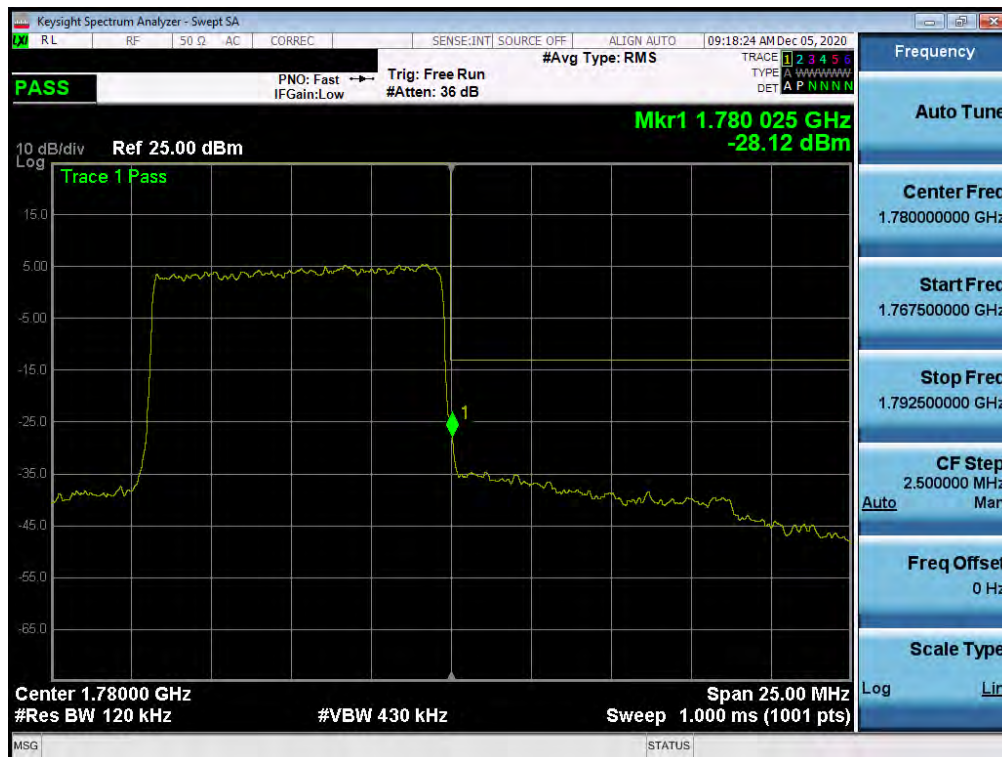
Plot 7-273. Upper Band Edge Plot (NR Band n66 – 10.0MHz - Full RB)
