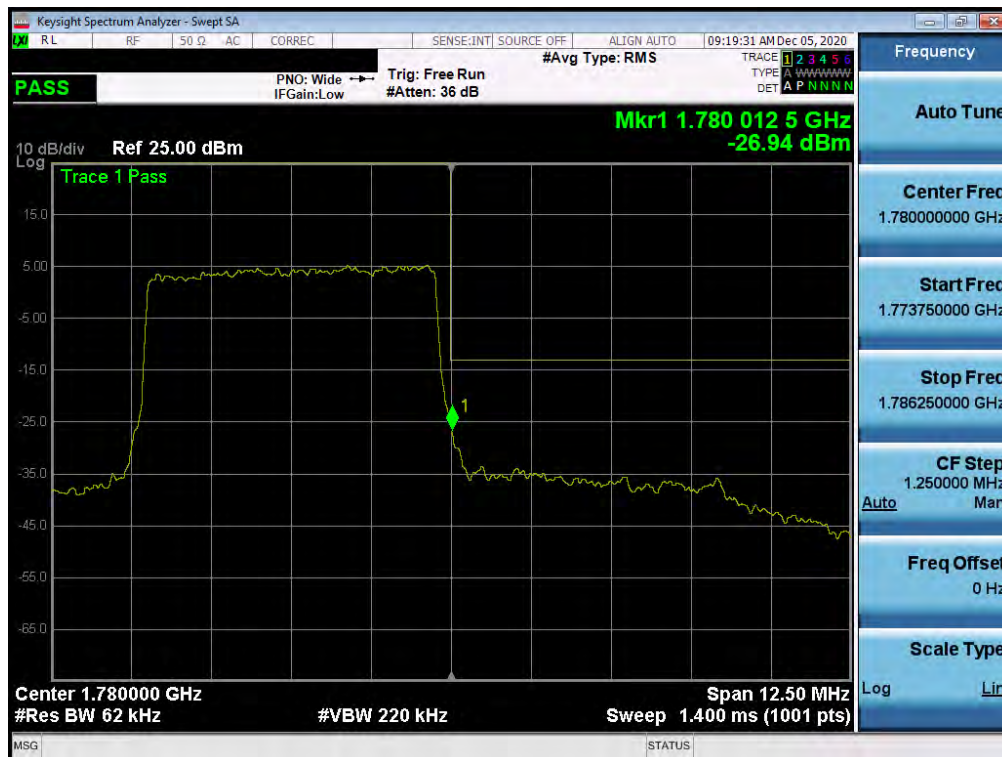
Plot 7-277. Upper Band Edge Plot (NR Band n66 – 5.0MHz - Full RB)
