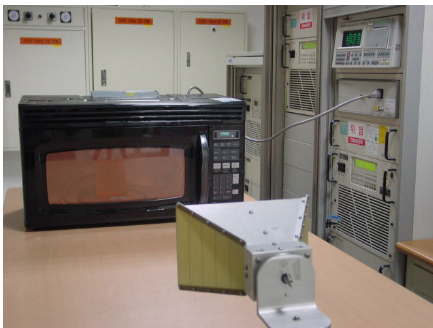
Fig. 2 Test Setup for Input power
