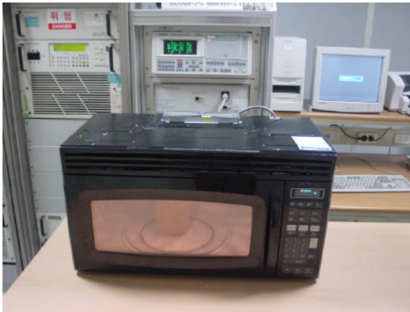
Fig.3 Test Setup for RF output power
