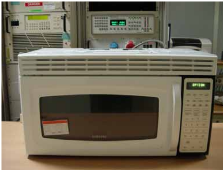
Fig.3 Test Setup for RF output power
