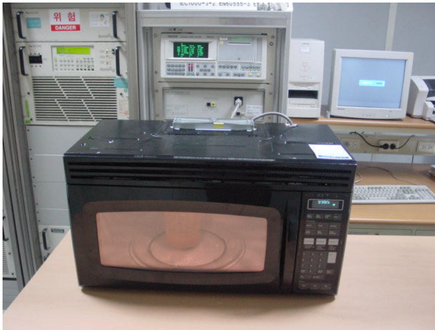
Fig.3 Test Setup for RF output power
