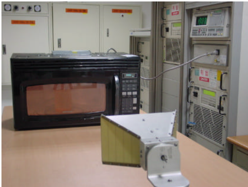
Fig. 2 Test Setup for Input power
