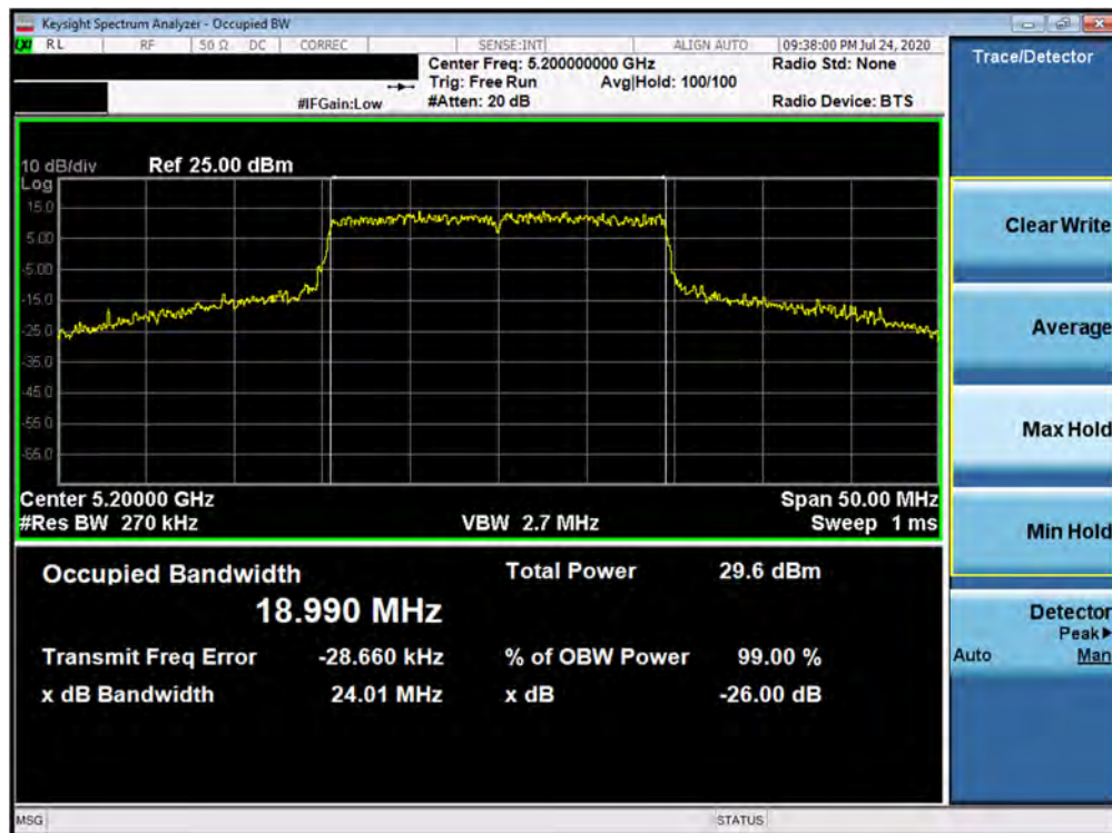
Plot 7-44. 26dB Bandwidth Plot ANT5 (20MHz BW 802.11ax – 242 Tones (UNII Band 1) – Ch. 40)
