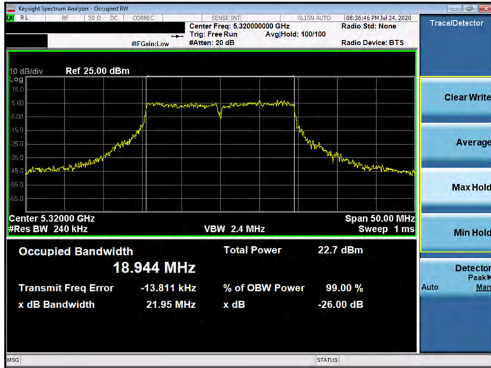
Plot 7-72. 26dB Bandwidth Plot ANT6 (20MHz BW 802.11ax – 242 Tones (UNII Band 2A) – Ch. 64)
