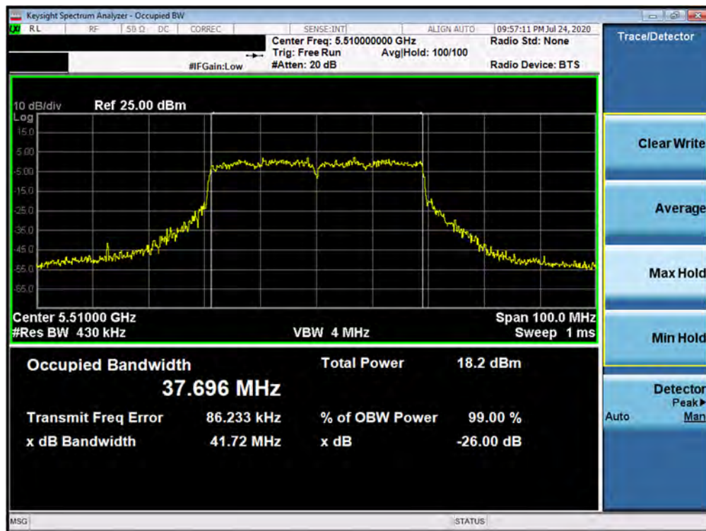
Plot 7-58. 26dB Bandwidth Plot ANT5 (40MHz BW 802.11ax – 484 Tones (UNII Band 2C) – Ch. 102)
