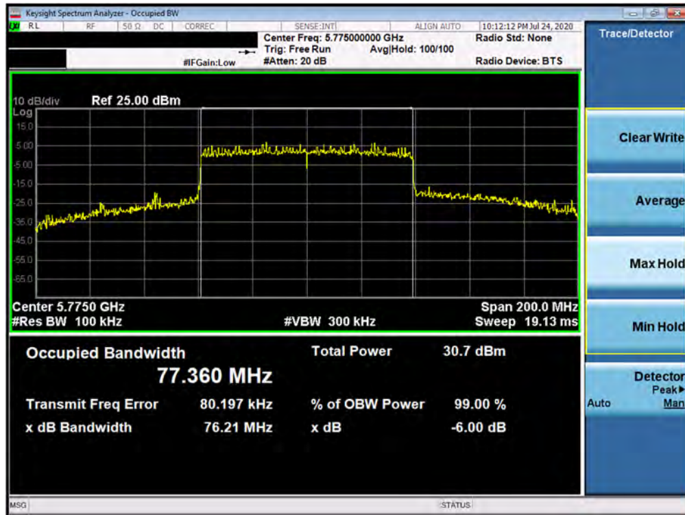
Plot 7-104. 6dB Bandwidth Plot ANT5 (80MHz BW 802.11ax – 996 Tones (UNII Band 3) – Ch. 155)
