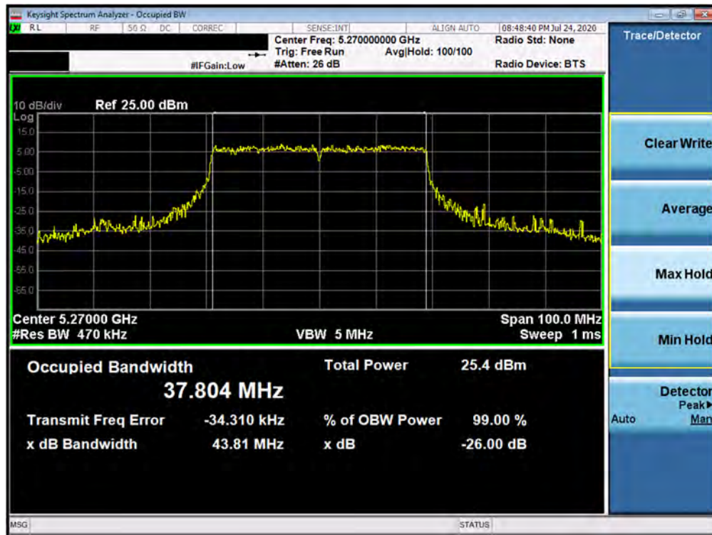
Plot 7-73. 26dB Bandwidth Plot ANT6 (40MHz BW 802.11ax – 484 Tones (UNII Band 2A) – Ch. 54)
