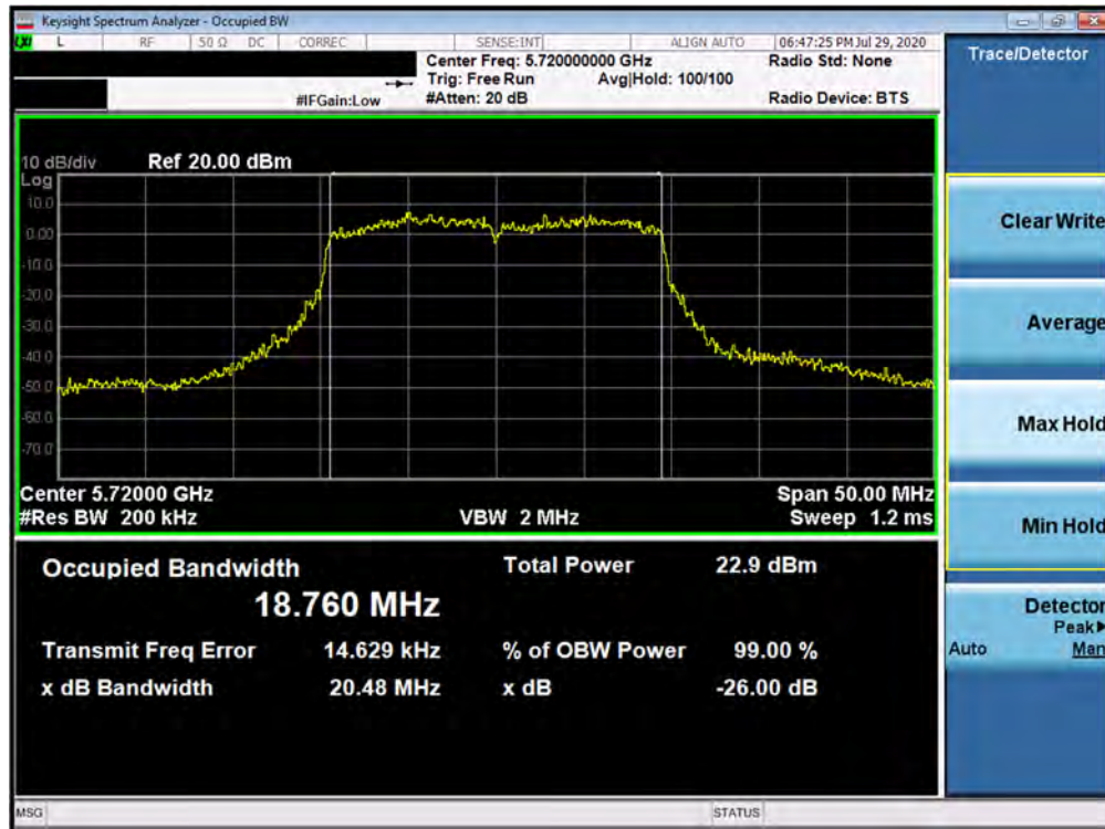
Plot 7-15. 26dB Bandwidth Plot ANT3 (20MHz BW 802.11ax – 242 Tones (UNII Band 2C) – Ch. 144)
