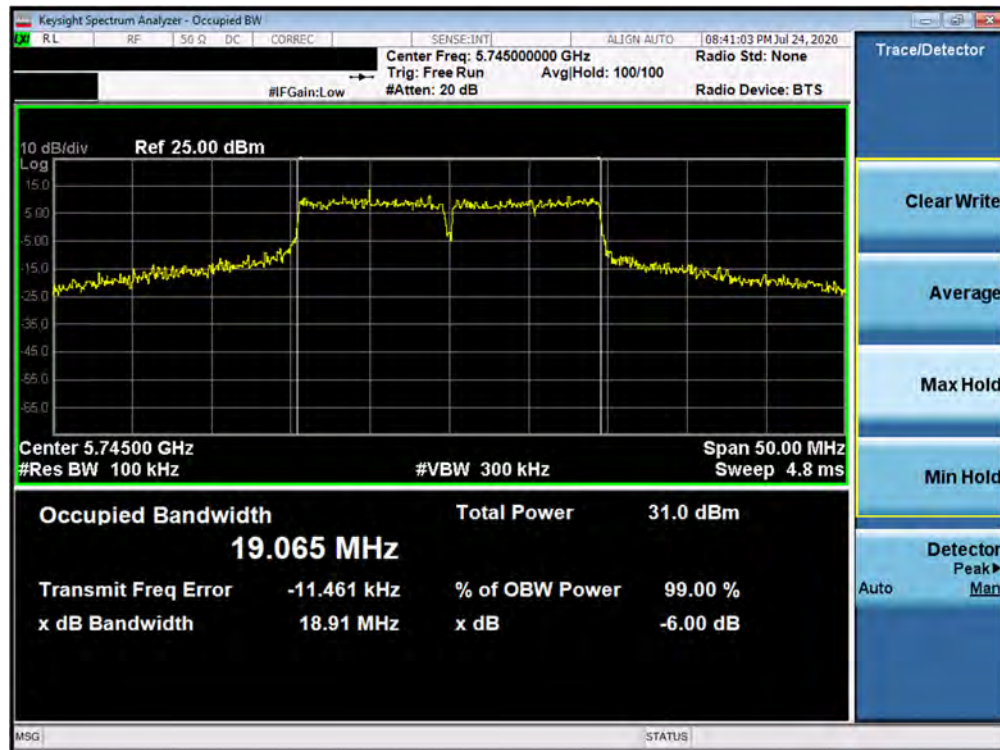
Plot 7-105. 6dB Bandwidth Plot ANT6 (20MHz BW 802.11ax – 242 Tones (UNII Band 3) – Ch. 149)
