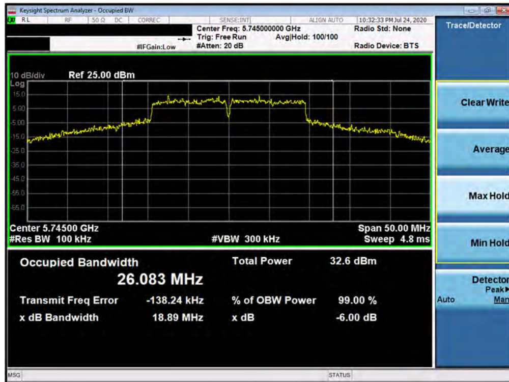
Plot 7-93. 6dB Bandwidth Plot ANT4 (20MHz BW 802.11ax – 242 Tones (UNII Band 3) – Ch. 149)
