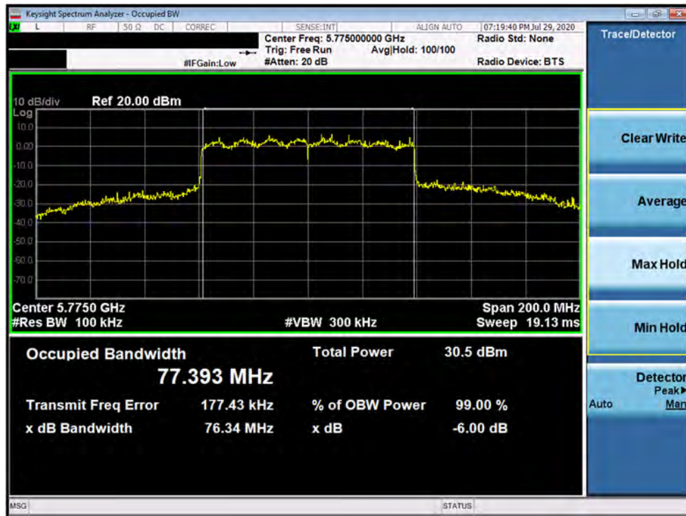
Plot 7-92. 6dB Bandwidth Plot ANT3 (80MHz BW 802.11ax – 996 Tones (UNII Band 3) – Ch. 155)
