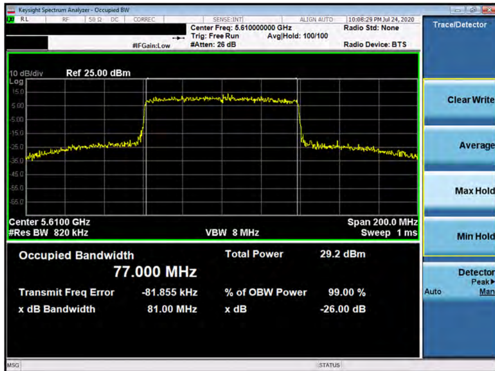
Plot 7-62. 26dB Bandwidth Plot ANT5 (80MHz BW 802.11ax – 996 Tones (UNII Band 2C) – Ch. 122)
