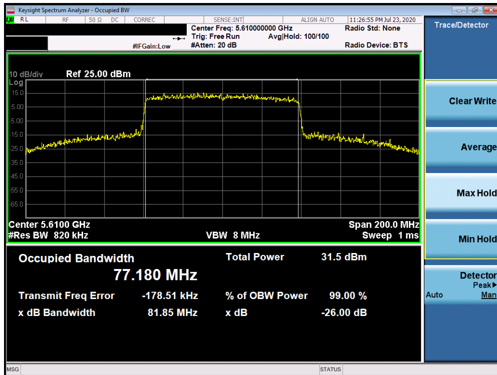
Plot 7-101. 26dB Bandwidth Plot ANT4 (80MHz BW 802.11ax (UNII Band 2C) – Ch. 122)
