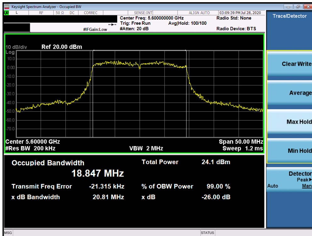
Plot 7-38. 26dB Bandwidth Plot ANT3 (20MHz BW 802.11ax (UNII Band 2C) – Ch. 120)
