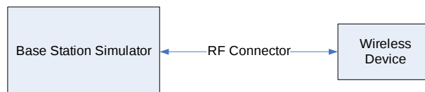
Figure 8-2 Power Measurement Setup
