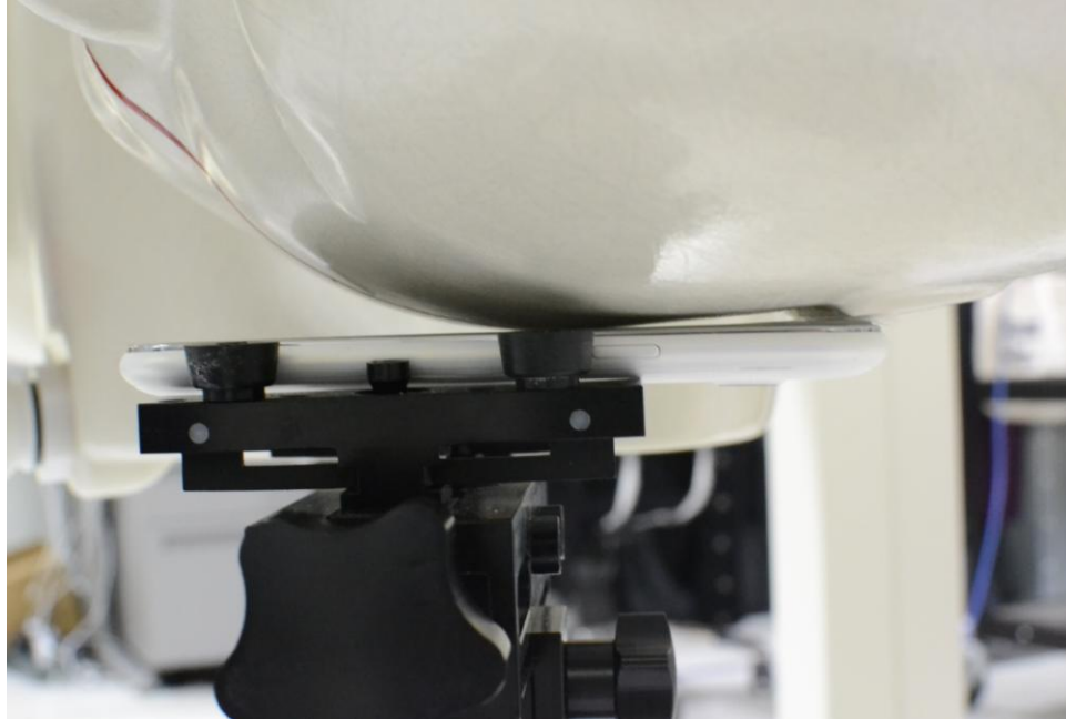
SAR Test Setup Photo 3: Left Cheek
