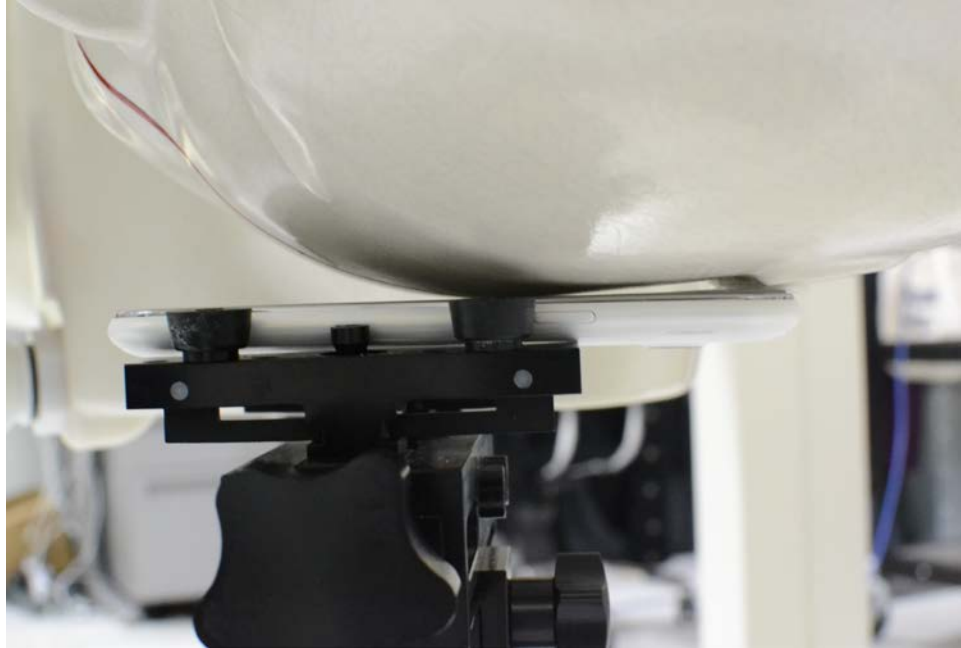
SAR Test Setup Photo 3: Left Cheek
