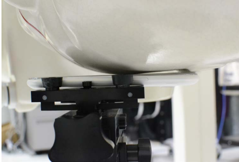
SAR Test Setup Photo 3: Left Cheek
