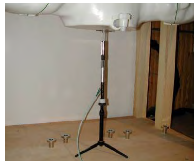
Figure 10-2 System Verification Setup Photo
