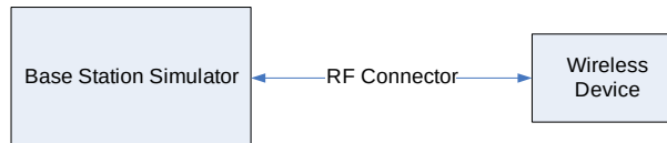
Figure 9-1 Power Measurement Setup
