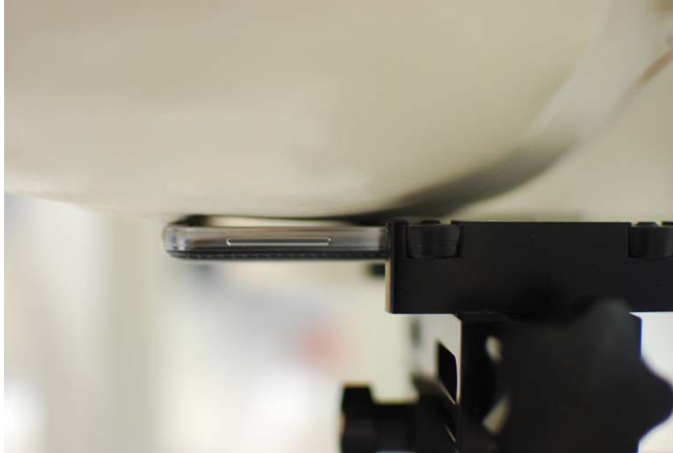
SAR Test Setup Photo 1 – Right Cheek
