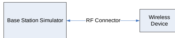
Figure 8-2 Power Measurement Setup
