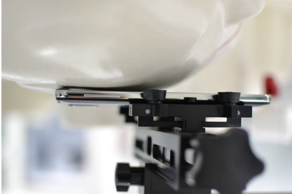
SAR Test Setup Photo 1 – Right Cheek
