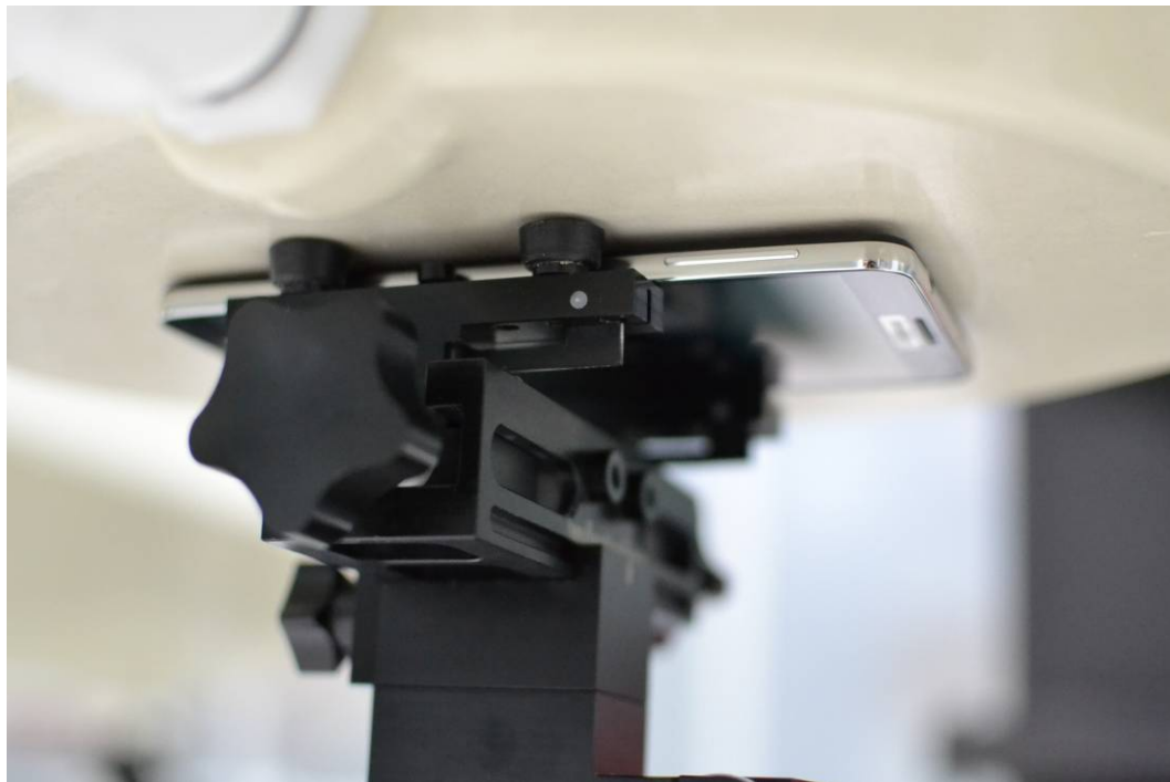
SAR Test Setup Photo 6 – Back at 0.0 cm
