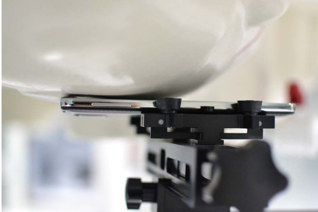
SAR Test Setup Photo 1 – Right Cheek
