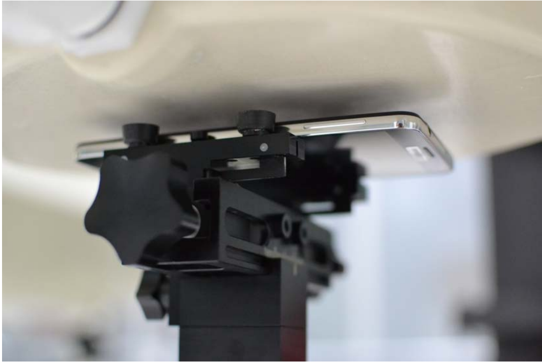
SAR Test Setup Photo 5– Back at 1.0 cm
