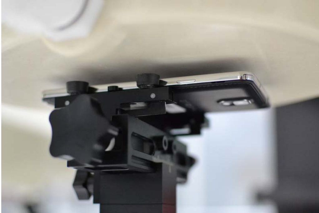
SAR Test Setup Photo 7 – Front at 1.0 cm
