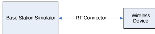
Figure 10-2 Power Measurement Setup
