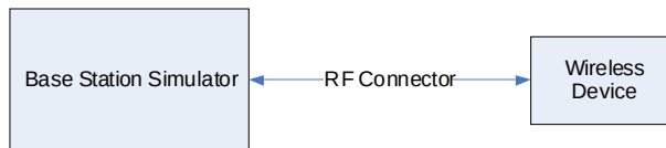
Figure 9-3 Power Measurement Setup
