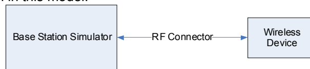
Figure 8-2 Power Measurement Setup
