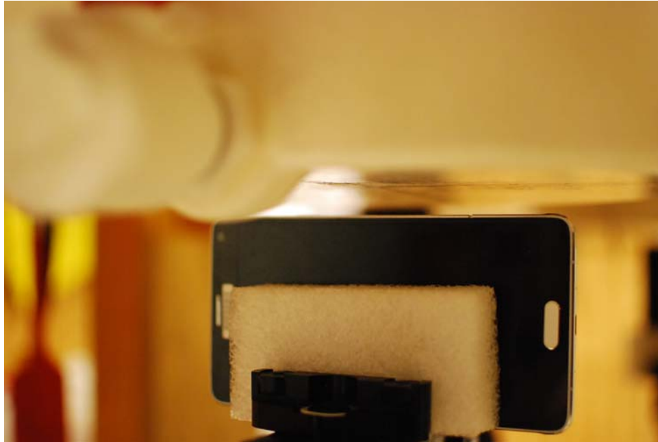
SAR Test Setup Photo 9: Right at 1.0 cm
