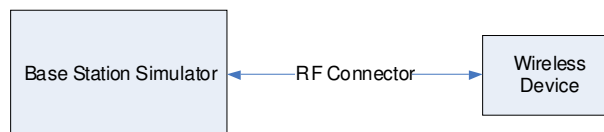
Figure 9-2 Power Measurement Setup
