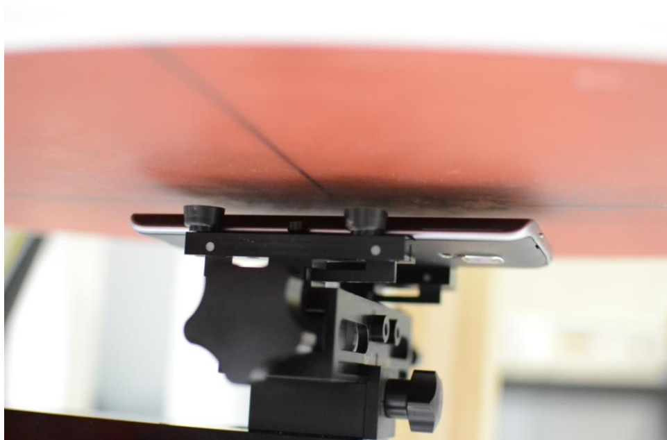
SAR Test Setup Photo 8 – Front Side at 1.0 cm (Hotspot)
