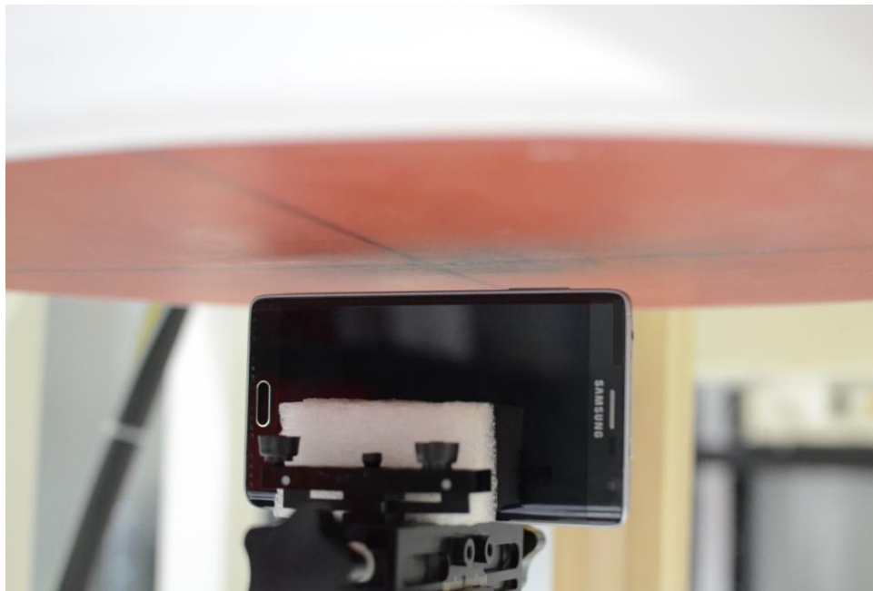
SAR Test Setup Photo 14 – Left Edge at 1.0 cm (Hotspot)
