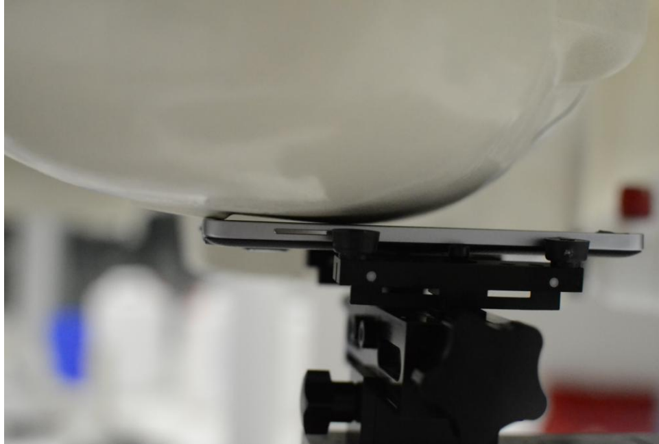
SAR Test Setup Photo 1 – Right Cheek
