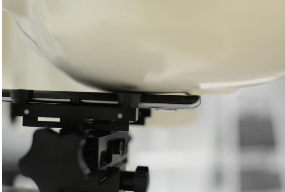
SAR Test Setup Photo 3 – Left Cheek
