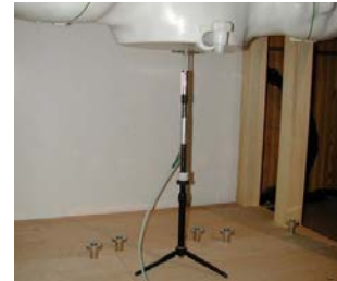
Figure 10-2 System Verification Setup Photo
