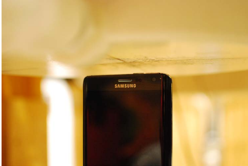
SAR Test Setup Photo 17 – Top Edge at 1.0 cm, Standard Back Cover
