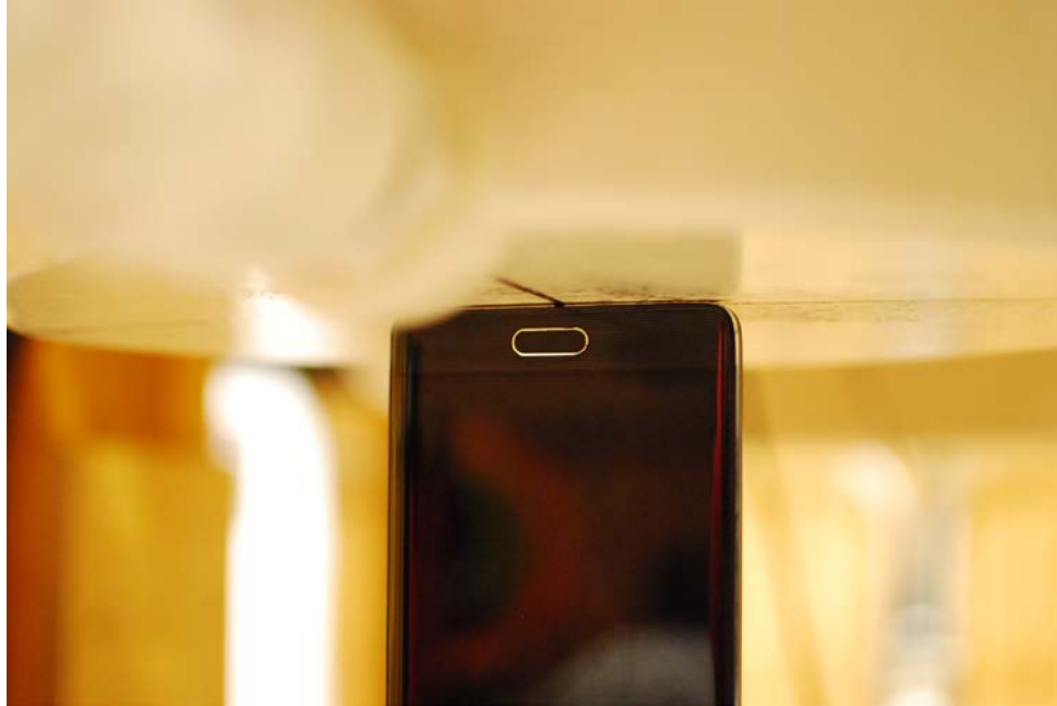
SAR Test Setup Photo 21 – Bottom Edge at 0.0 cm, Standard Back Cover
