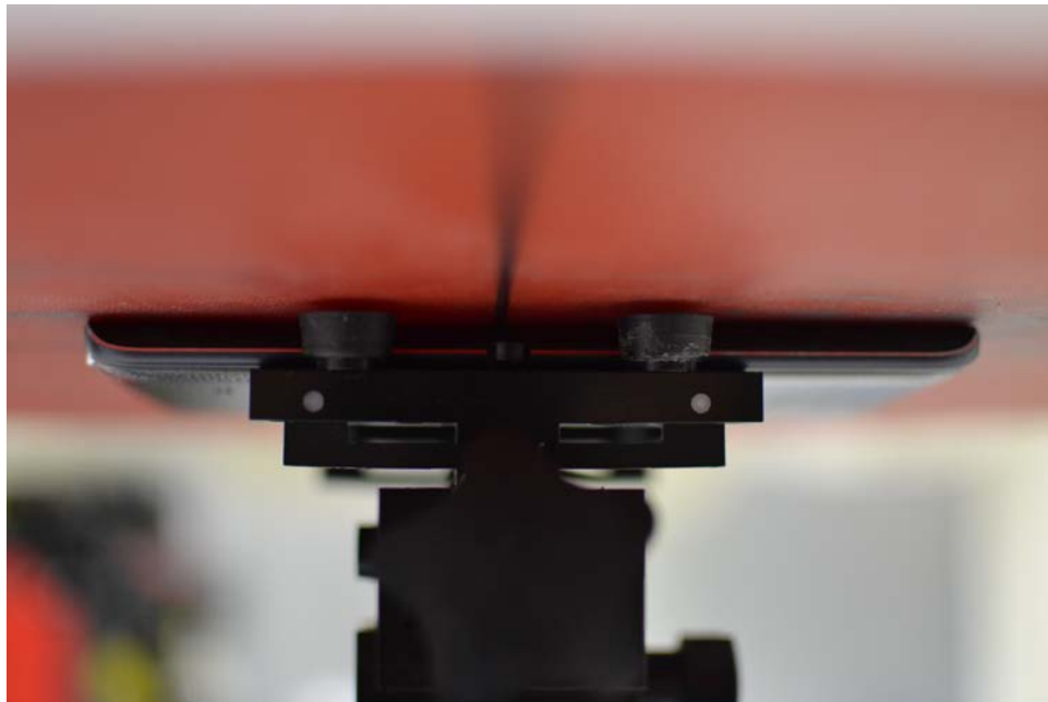
SAR Test Setup Photo 16 – Front Side at 0.0 cm, Wireless Charging Cover
