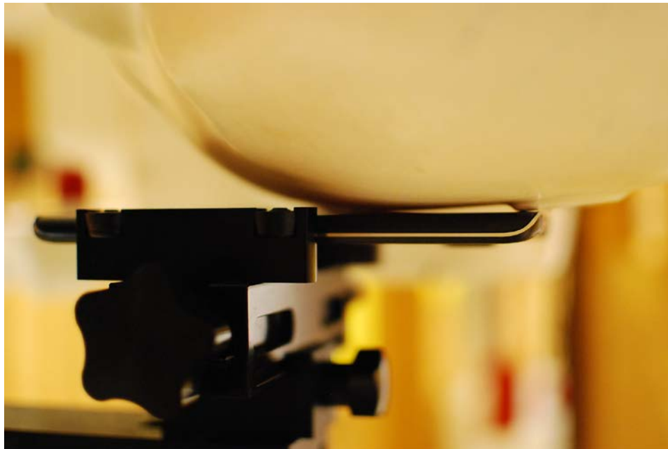
SAR Test Setup Photo 4 – Left Cheek, Standard Back Cover
