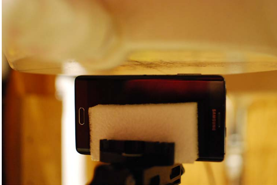
SAR Test Setup Photo 25 – Left Edge at 1.0 cm, Standard Back Cover
