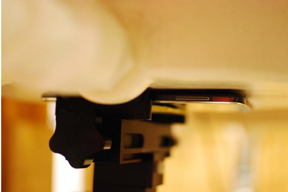
SAR Test Setup Photo 11 – Back Side at 0.0 cm, Standard Back Cover
