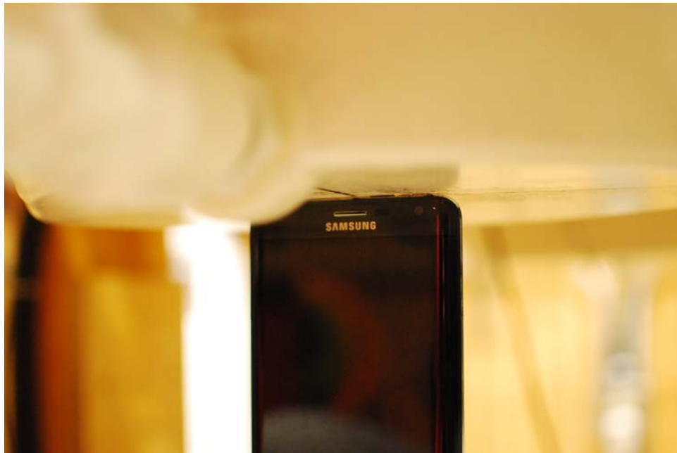
SAR Test Setup Photo 18 – Top Edge at 0.0 cm, Standard Back Cover
