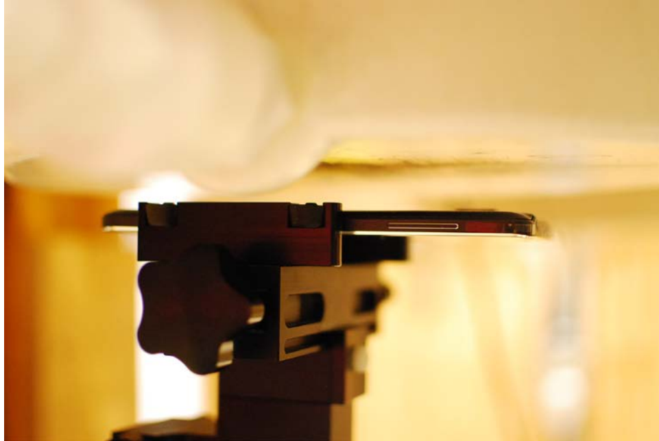
SAR Test Setup Photo 7 – Back Side at 1.5 cm, Standard Back Cover
