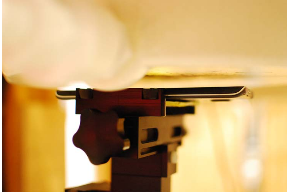
SAR Test Setup Photo 13 – Front Side at 1.0 cm, Standard Back Cover
