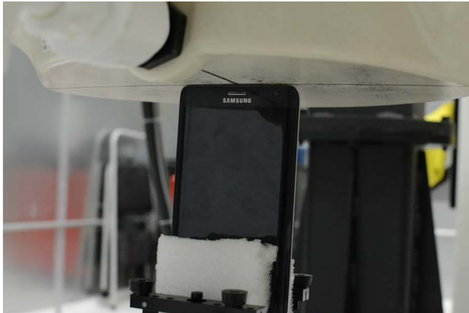
SAR Test Setup Photo 21 – Top Edge at 0.0 cm
