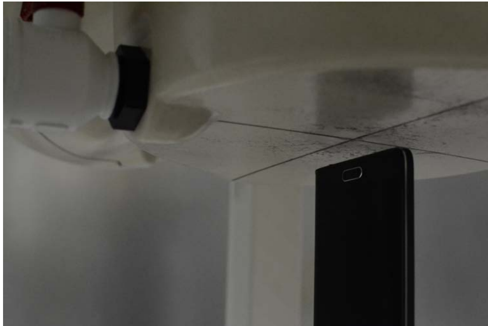
SAR Test Setup Photo 23 – Bottom Edge at 1.0 cm with Wireless Charging Cover
