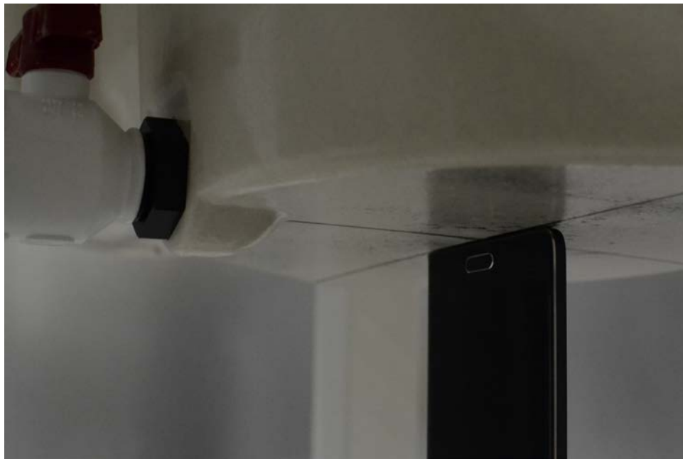
SAR Test Setup Photo 26 – Bottom Edge at 0.0 cm with Wireless Charging Cover
