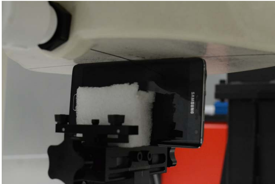
SAR Test Setup Photo 30 – Left Edge at 0.0 cm
