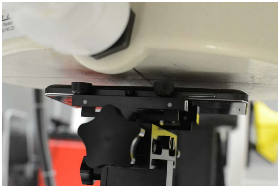
SAR Test Setup Photo 10 – Back Side at 1.0 cm with Wireless Charging Cover
