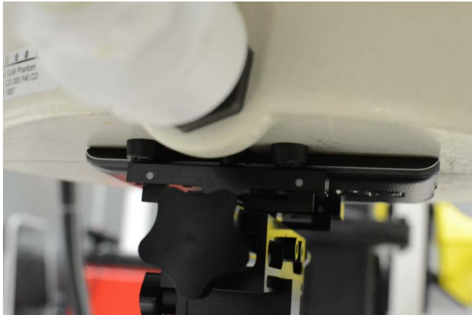
SAR Test Setup Photo 19 – Front Side at 0.0 cm with Wireless Charging Cover
