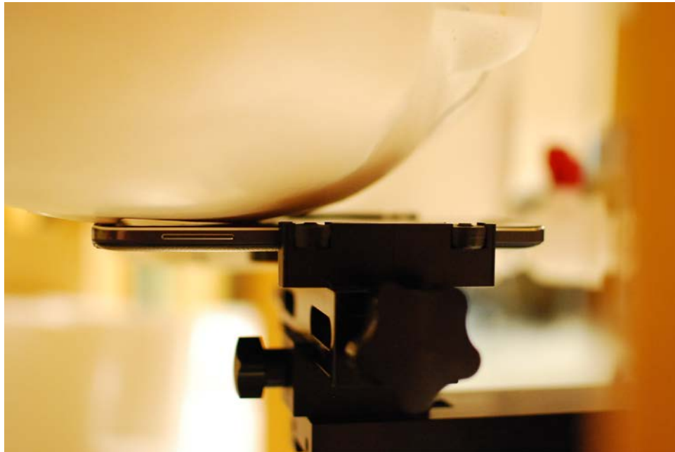
SAR Test Setup Photo 1 – Right Cheek
