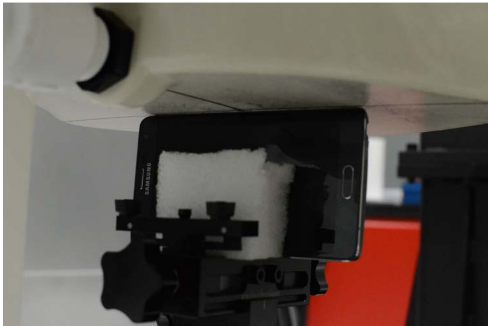
SAR Test Setup Photo 28 – Right Edge at 0.0 cm
