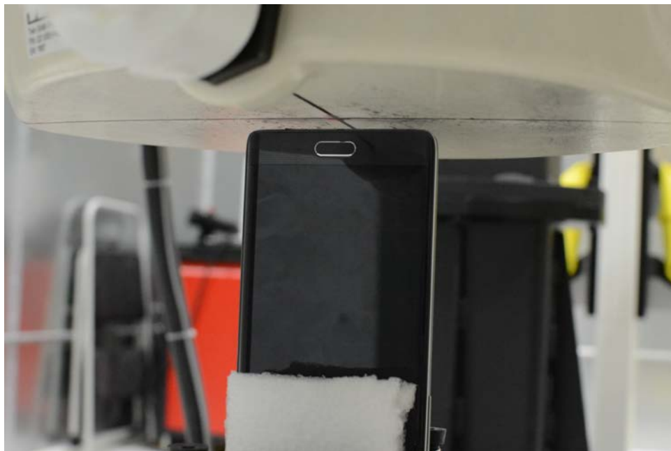
SAR Test Setup Photo 24 – Bottom Edge at 0.4 cm
