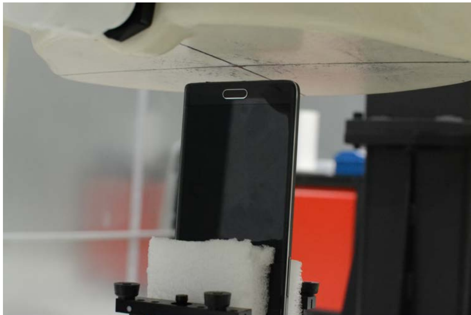
SAR Test Setup Photo 22 – Bottom Edge at 1.0 cm
