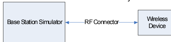
Figure 9-3 Power Measurement Setup
