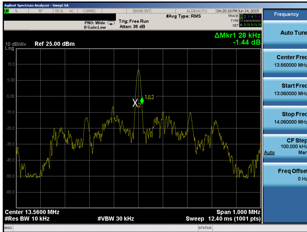
Figure 7-2. 20dB Bandwidth Plot
