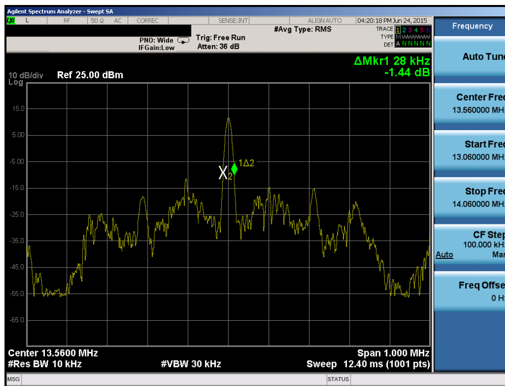
Figure 7-2. 20dB Bandwidth Plot
