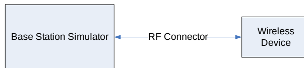
Figure 9-3 Power Measurement Setup
