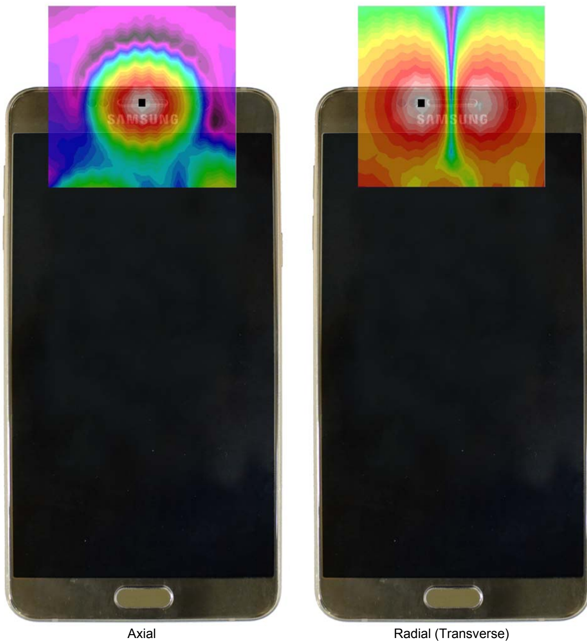
Figure 13-3 T-Coil Scan Overlay Magnetic Field Distributions
