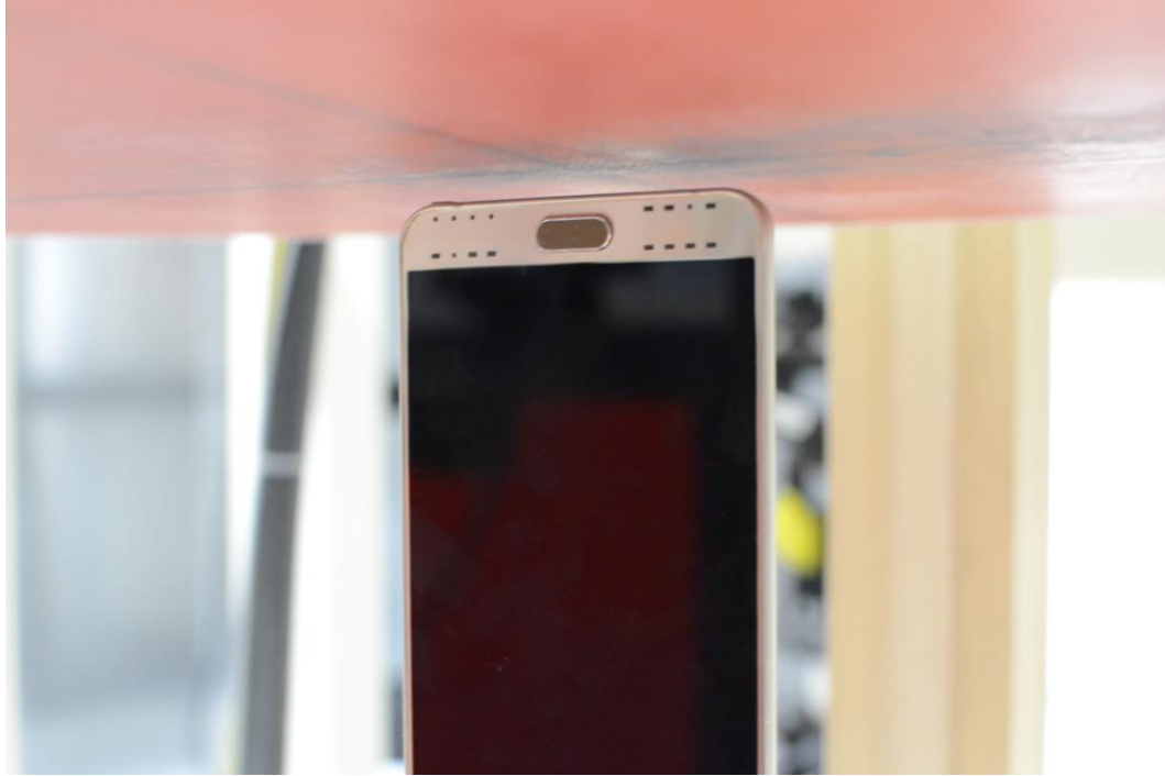
SAR Test Setup Photo 15– Bottom Edge at 0.5 cm (Extremity)
