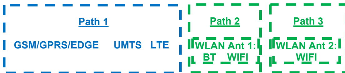
Figure 1-1 Simultaneous Transmission Paths
