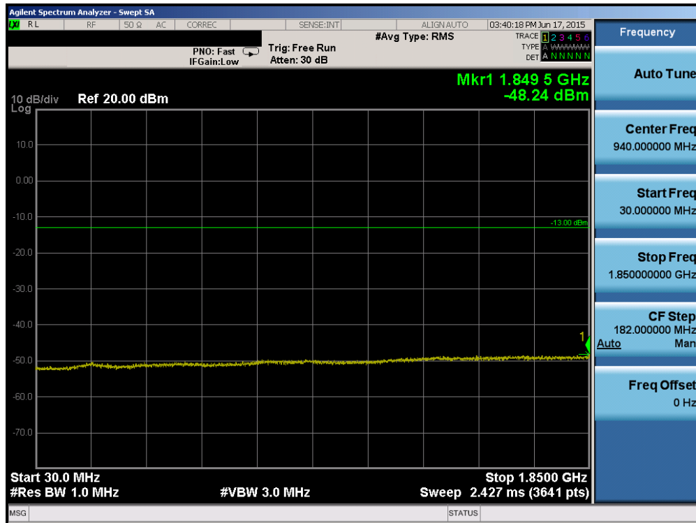
Plot 6-47. Conducted Spurious Plot (PCS WCDMA Mode – Ch. 9400)
