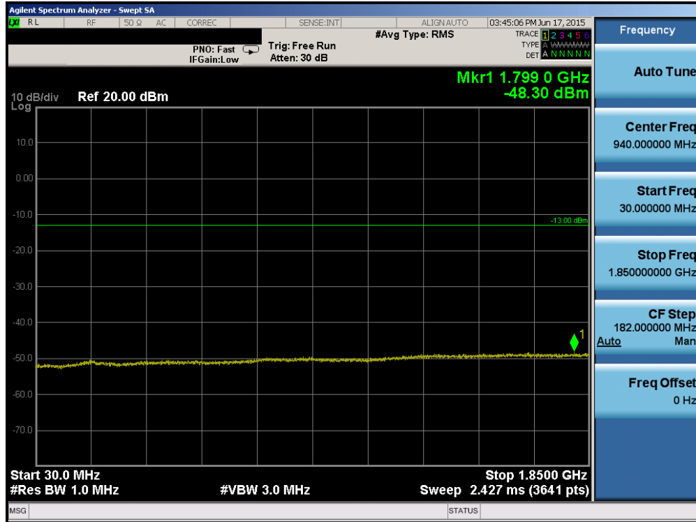
Plot 6-50. Conducted Spurious Plot (PCS WCDMA Mode – Ch. 9538)
