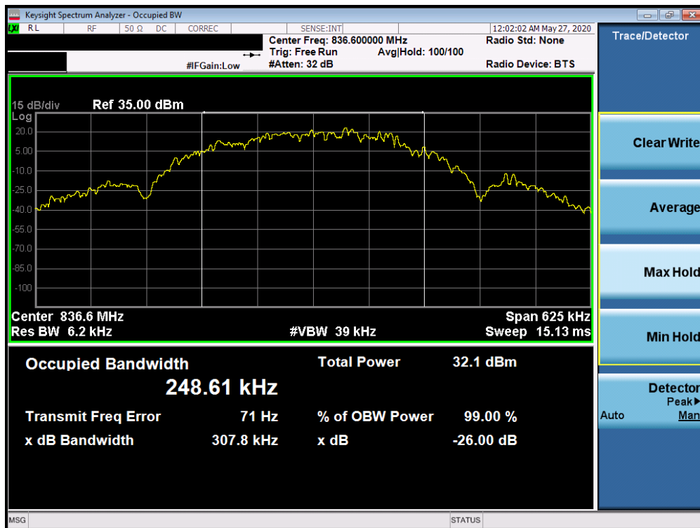
Plot 7-2. Occupied Bandwidth Plot (EDGE850 Mode)
