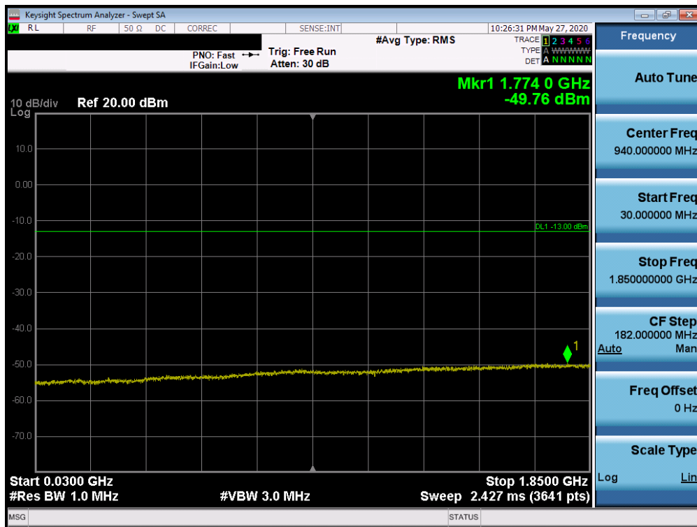
Plot 7-57. Conducted Spurious Plot (PCS WCDMA Mode - Mid Channel)
