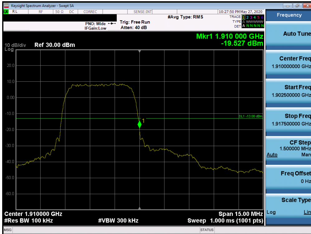
Plot 7-78. Band Edge Plot (PCS WCDMA Mode - High Channel)
