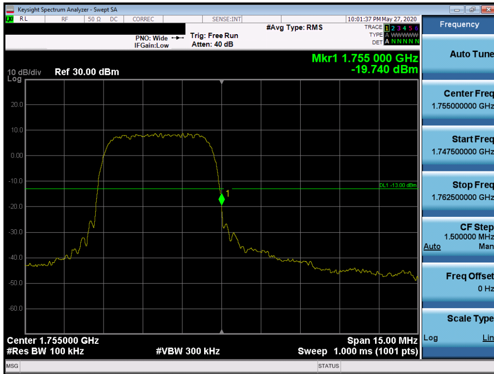
Plot 7-75. Band Edge Plot (AWS WCDMA Mode - High Channel)
