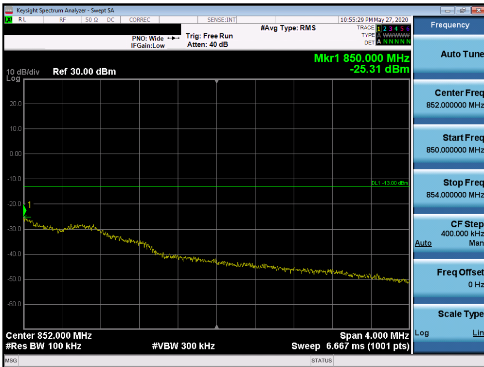
Plot 7-70. 4MHz Span Plot (Cellular CDMA Mode - High Channel)
