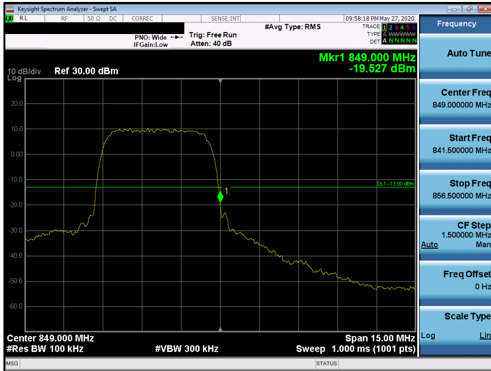
Plot 7-72. Band Edge Plot (Cellular WCDMA Mode - High Channel)
