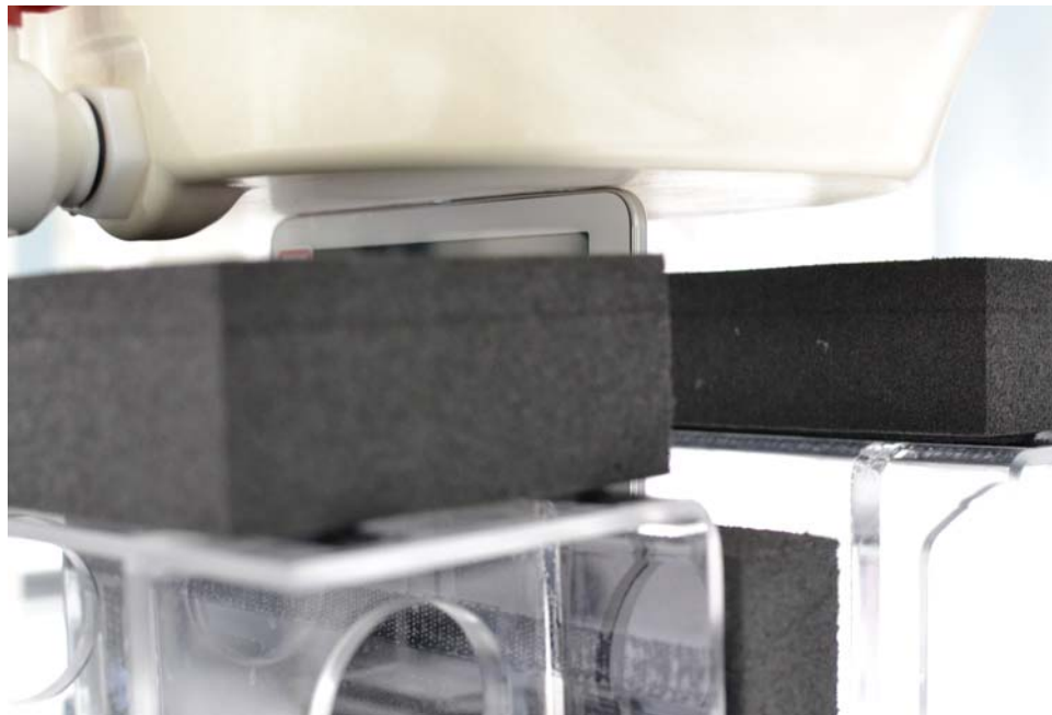
SAR Test Setup Photo 4: Right Edge at 0 mm
