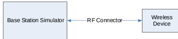
Figure 8-1 Power Measurement Setup
