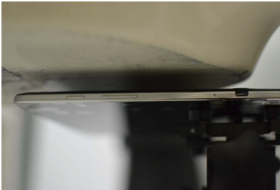
SAR Test Setup Photo 2 – Back side at 1.3 cm
