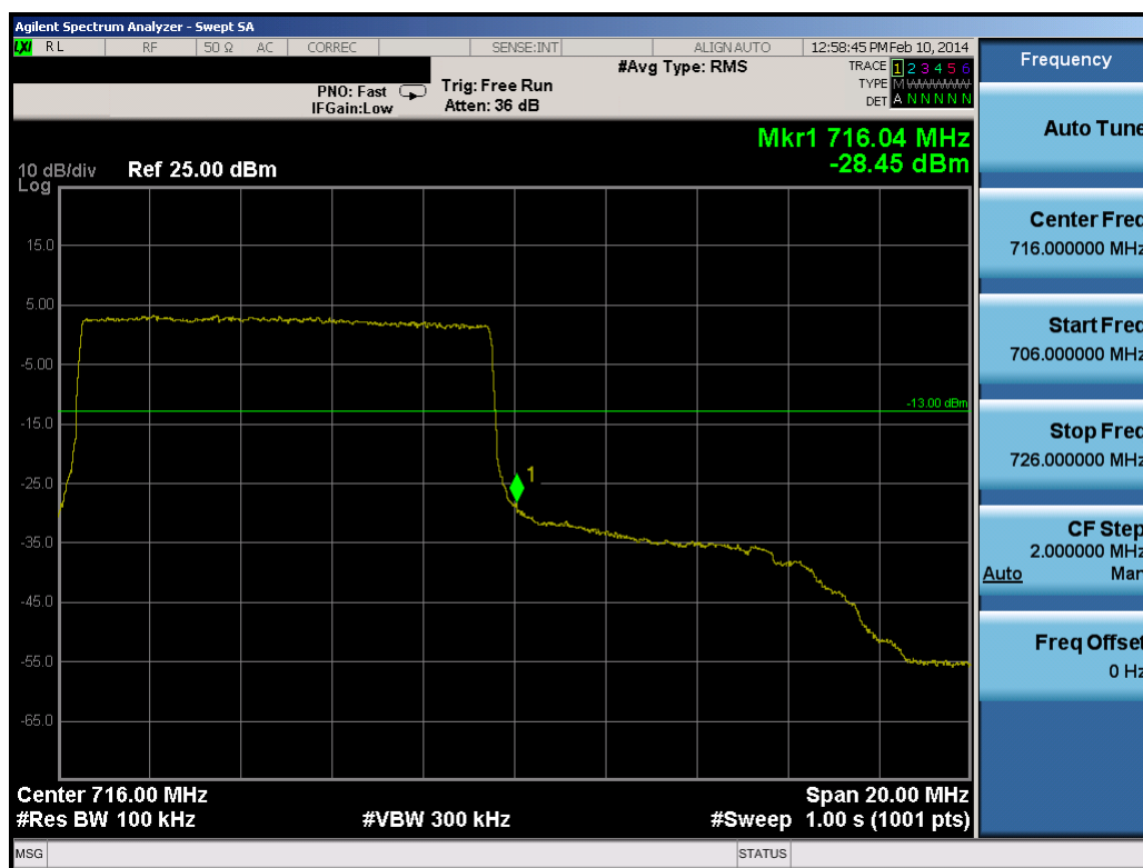
Plot 7-20. Upper Band Edge Plot (10.0MHz QPSK – RB Size 50)
