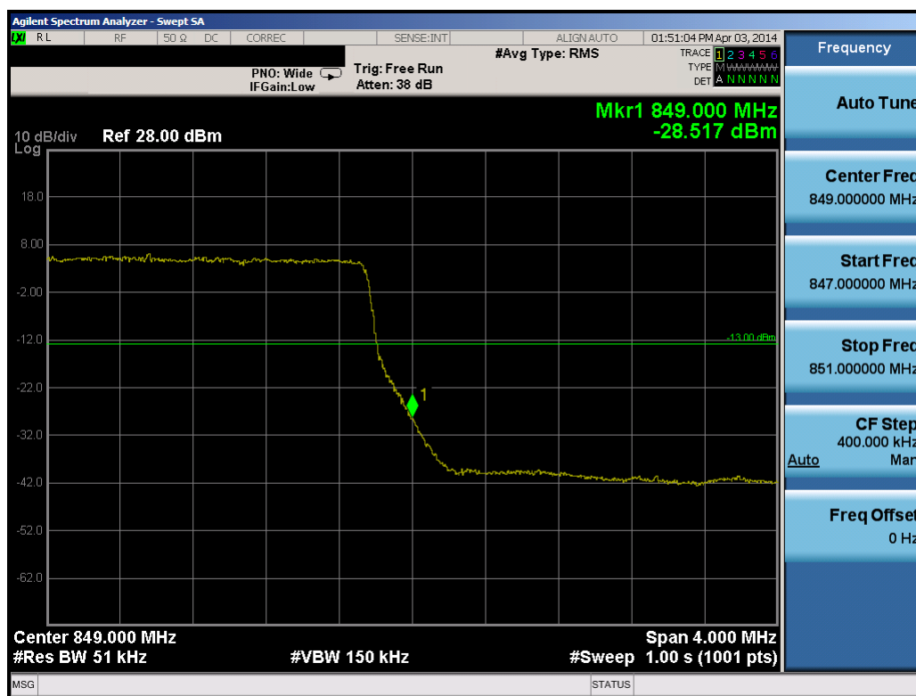
Plot 8-18. Upper Band Edge Plot (5.0MHz QPSK – RB Size 25)
