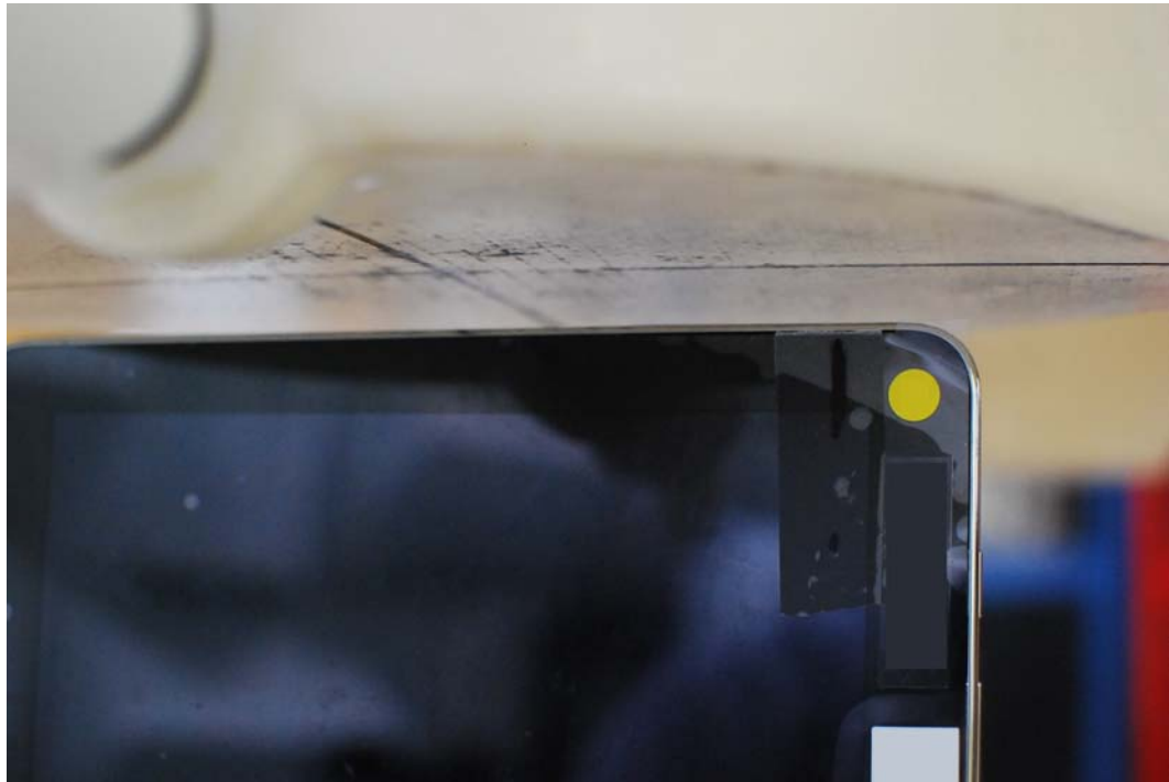
SAR Test Setup Photo 5: Left at 20 mm
