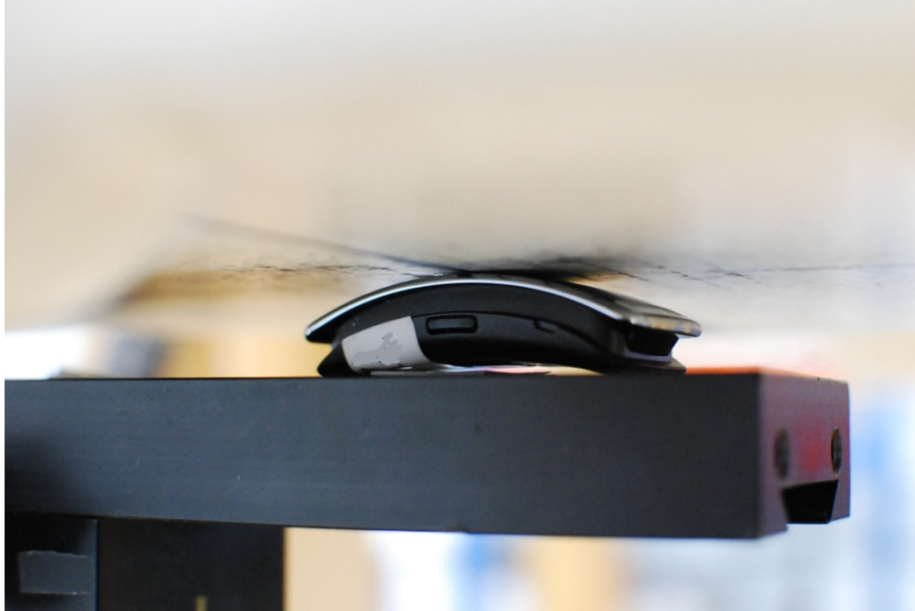
SAR Test Setup Photo 3: Front Side at 0.0 cm
