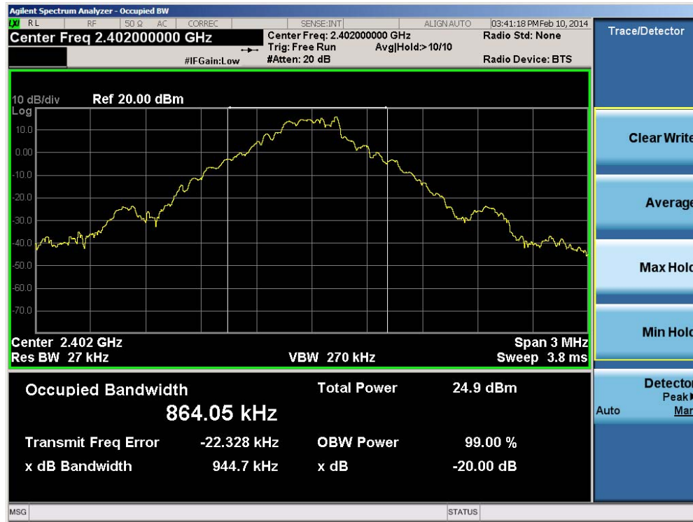
Plot 6-1. 20dB Bandwidth Plot (Bluetooth, 1Mbps – Ch. 0)
