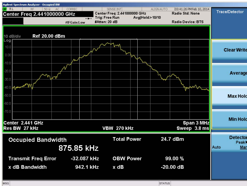
Plot 6-2. 20dB Bandwidth Plot (Bluetooth, 1Mbps – Ch. 39)
