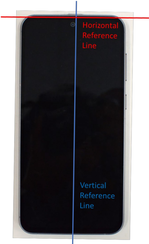
SAR Test Setup Photo 17 – Reference Lines
