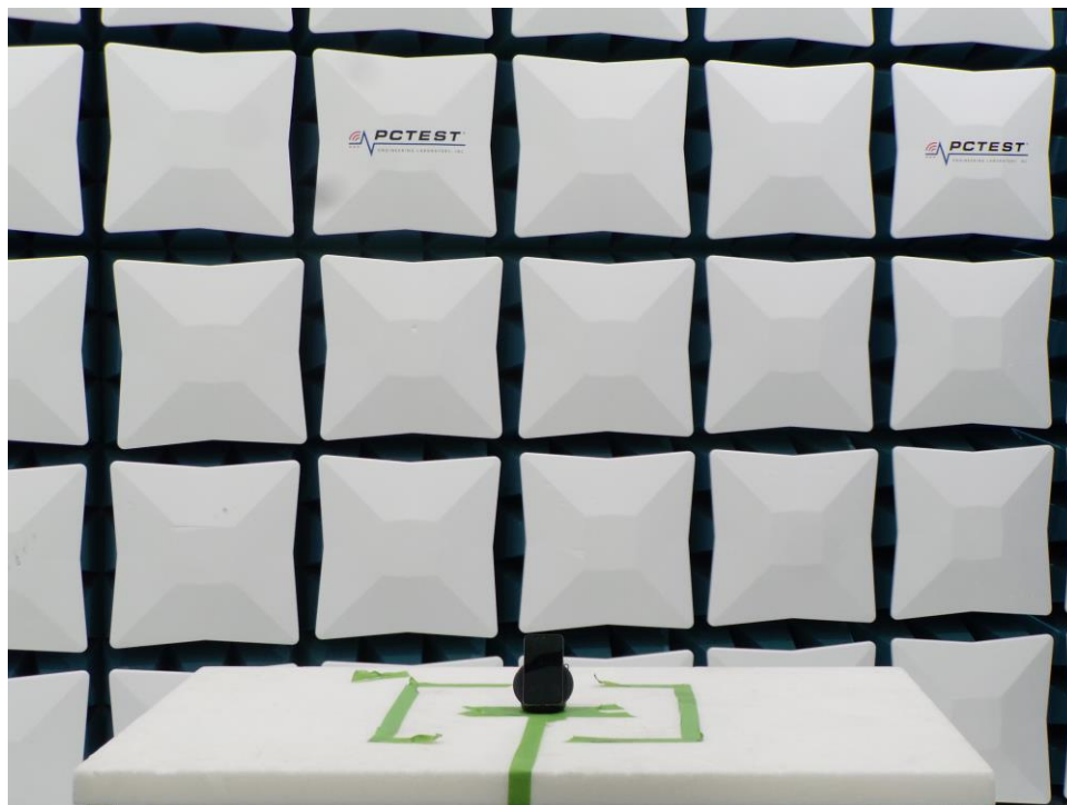
Figure 10. Test Setup – WCP Position – 30MHz-1GHz
