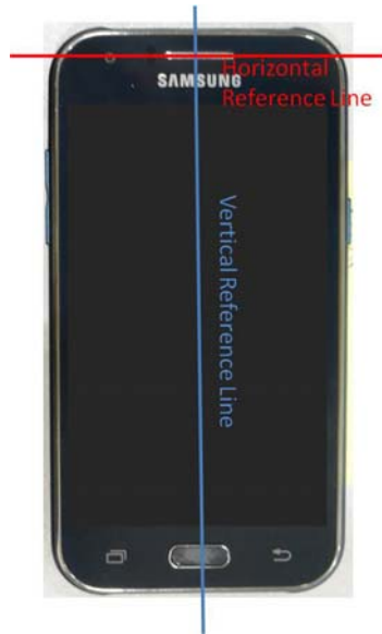
SAR Test Setup Photo 9: Horizontal and Vertical Reference Lines
