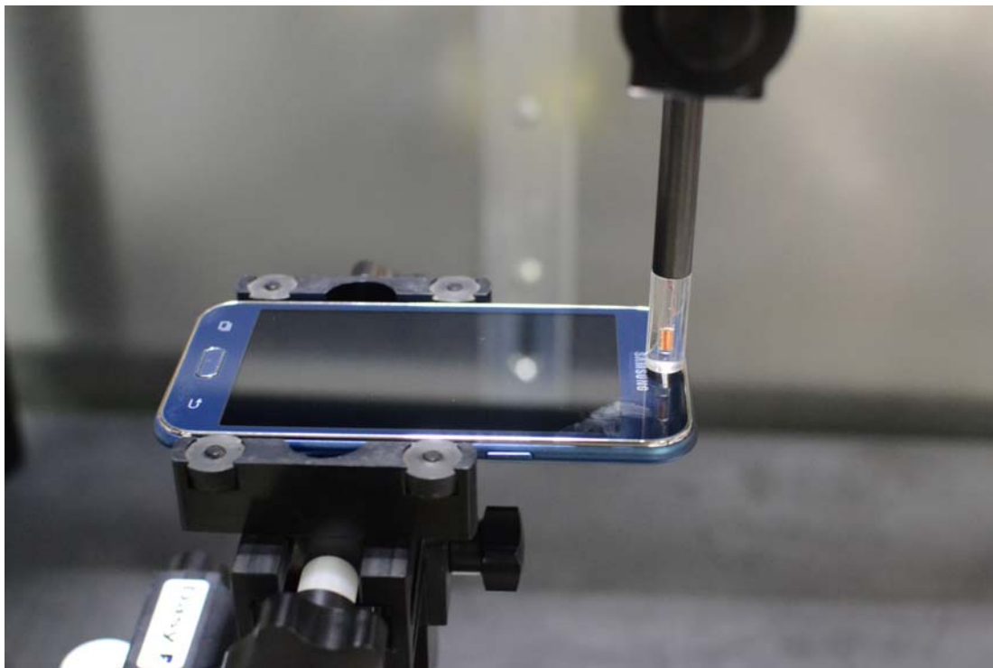
Figure 12-1 Test Setup for Wireless Device
