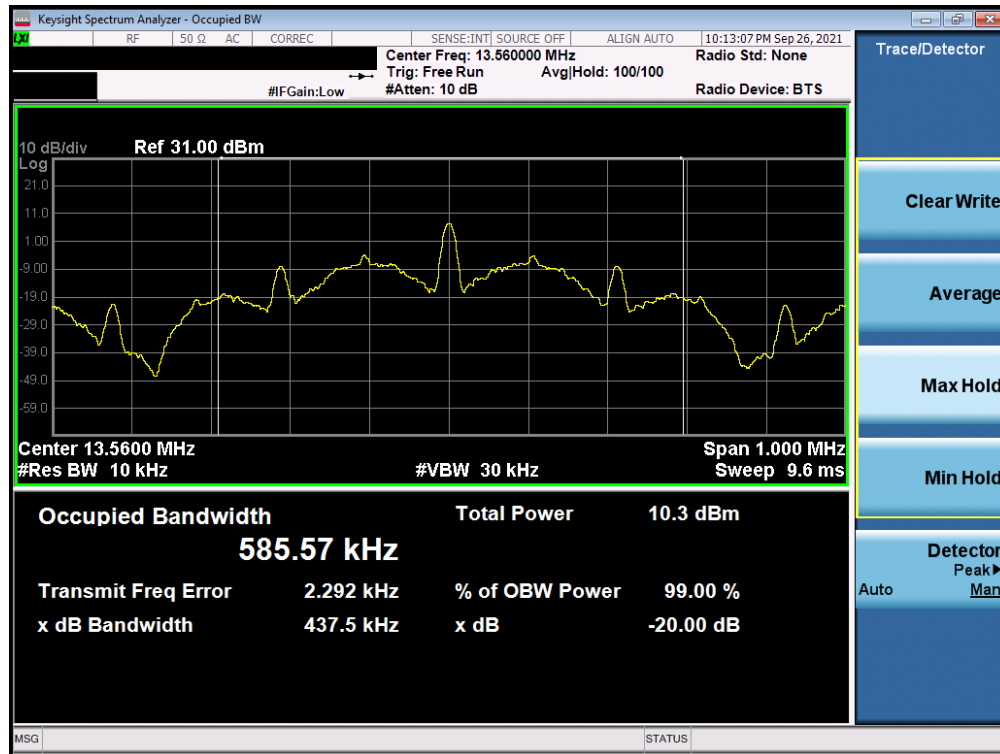
Plot 7-1. 20dB and 99% Bandwidth Plot
