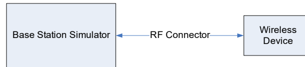
Figure 9-3 Power Measurement Setup
