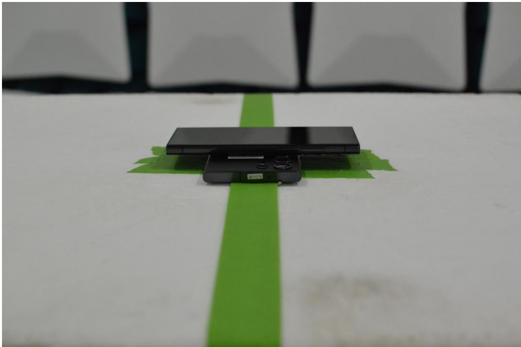
Figure 14. Test Setup – WPT Position – 1GHz-18GHz
