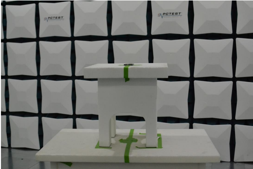
Figure 2. Test Setup – X Position – 1GHz-18GHz
