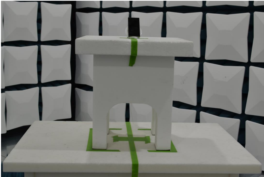
Figure 11. Test Setup – WCP Position – 1GHz-40GHz
